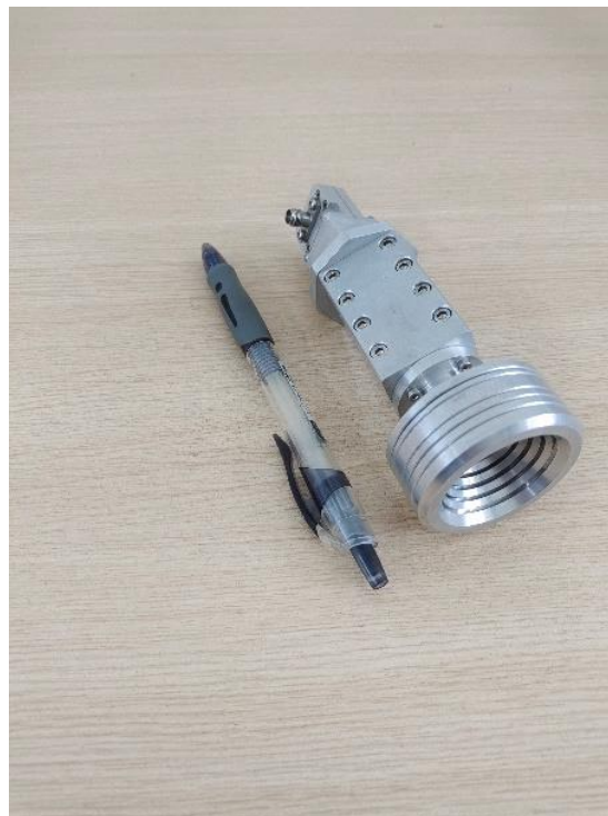
Figure 17. Photographs of the fabricated CP conical corrugated horn antenna.
