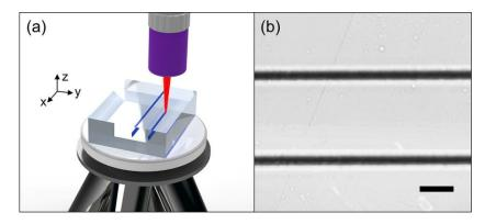
**Figure 1.** (a) The schematic diagram of femtosecond laser processing. Coordinate axes are defined here. (b) The microscope image of the processed KTN sample ( $x \times y$  facet). The scale bar in (b) is 20  $\mu$ m.
