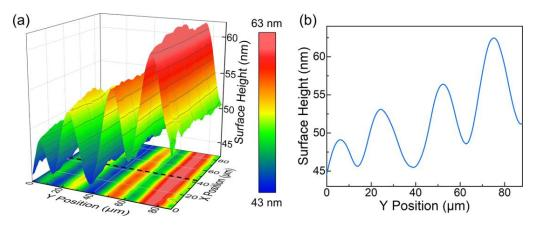
**Figure 4.** (a) Three-dimensional contour map of the femtosecond laser processed region on the  $x \times y$  facet. The raw data are releveled according to other unprocessed regions of the sample surface. (b) The height profile along the black dotted line in (a).
