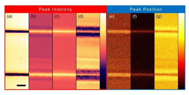
**Figure 3.** Two-dimensional spatial distributions of the Raman spectra representing (a-d) peak intensities and (e-g) peak positions obtained at room temperature. Channel details can be found in Table 1. The scale bar is 10  $\mu$ m.
