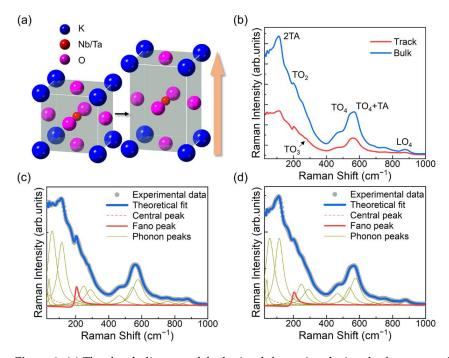
**Figure 2.** (a) The sketch diagram of the lattice deformation during the femtosecond laser processing. (b) The Raman scattering spectra of the femtosecond laser induced track (red line, and the bulk material (blue line), respectively. (c) Corresponding fitting curves of the track, and (d) the bulk material, respectively.
