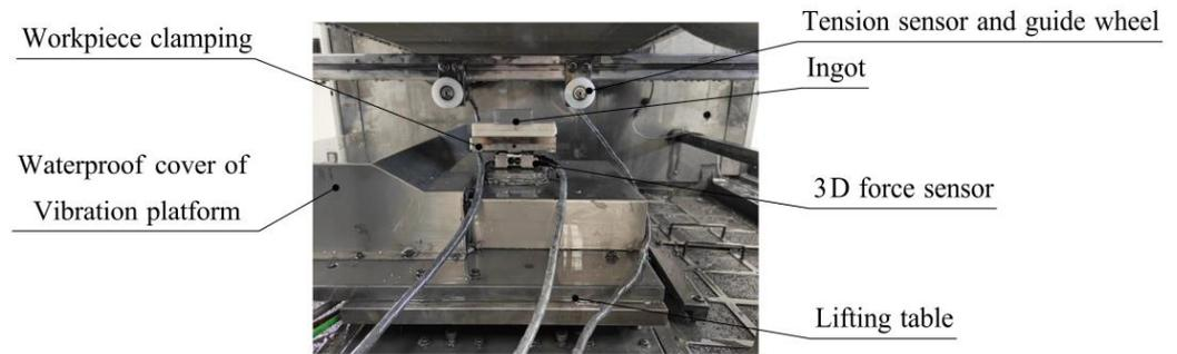
Figure 7. Measurement of experimental parameters.
