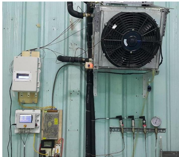
Figure 6. A V-finned tube evaporator for the CO<sub>2</sub> air conditioning system.
