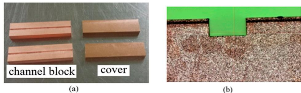
**Figure 9.** (a) Copper channel blocks and corresponding covers. (b) Cross-section of the channel.
