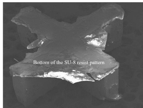
**Figure 5.** A thin resist layer on the bottom of the SU-8 resist pattern undeveloped in the developer solution, because it cross-linked in the soft bake at temperature exceeding 130  $^{\circ}\text{C}$ .
