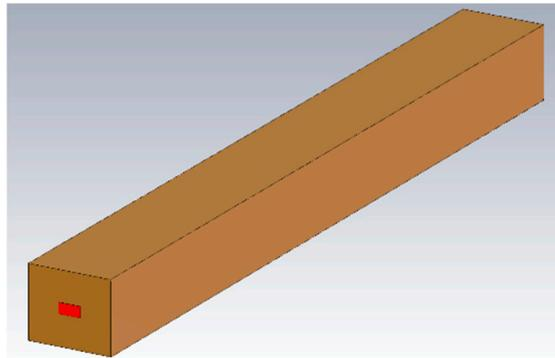
**Figure 14.** The model of the WR2.8 waveguide used in the CST calculation. The copper conductivity was set as  $2.95 \times 10^7 \text{ S/m}$  in calculation.
