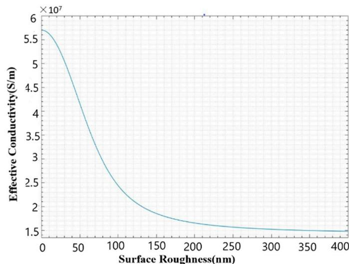
**Figure 13.** The effect of surface roughness on effective conductivity values at 340 GHz, showing the relative decrease in conductivity as a function of surface roughness.
