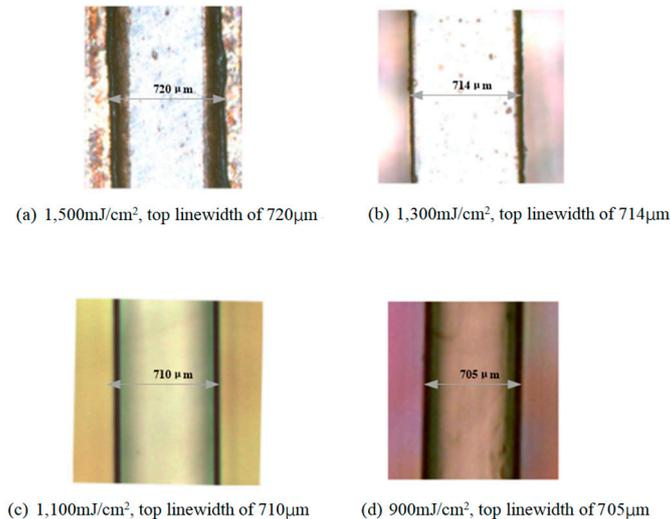
**Figure 6.** SU-8 resist patterns obtained by various exposure dosages and corresponding top linewidth.
