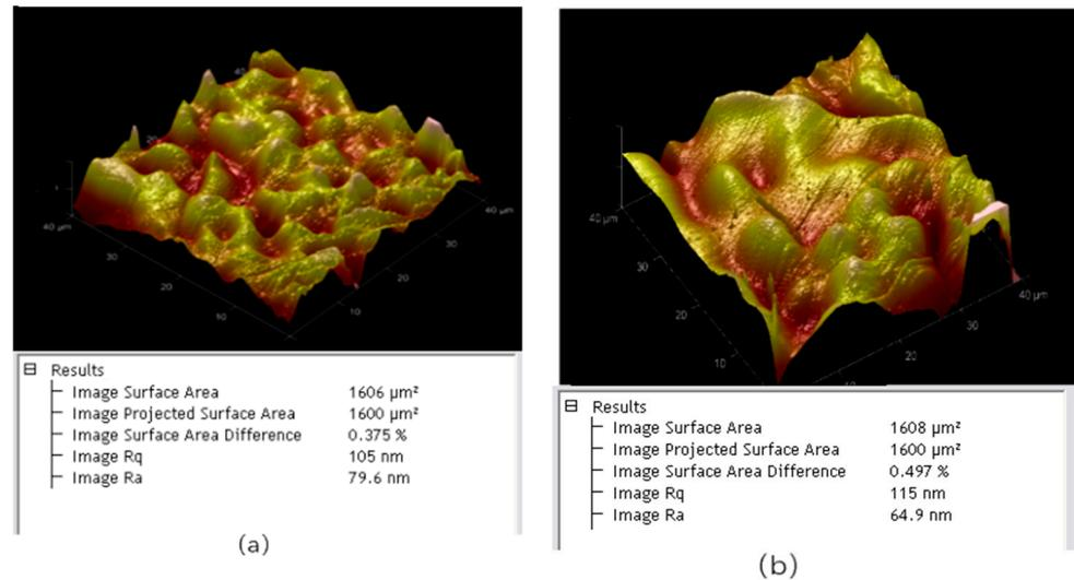
**Figure 12.** Testing sidewall roughness of the channel at two different spots with atomic force microscopy. (a) The sidewall roughness is 79.6 nm at one spot ( $R_a = 79.6$  nm). (b) The sidewall roughness is 64.9 nm at another spot ( $R_a = 64.9$  nm).
