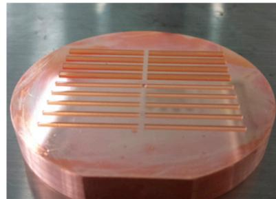
**Figure 7.** Optical microscope photograph of 18 SU-8 molds with optimum parameters on a copper disc: 8 SU-8 molds above for WR2.8 and 10 molds below for WR1.5.
