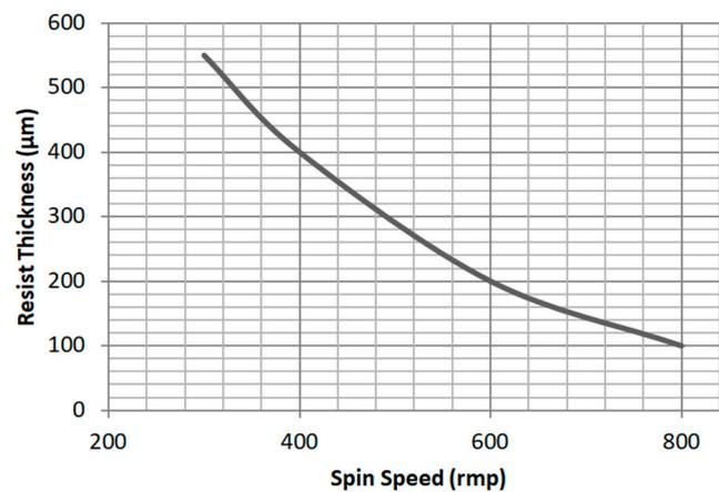
**Figure 4.** SU-8 2150 spin speed versus thickness. A spin speed of 400 rpm generates a 400  $\mu\text{m}$ -thick SU-8 resist film.
