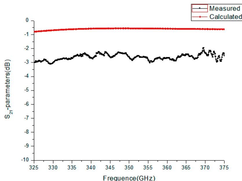
**Figure 15.** The experimentally measured  $S_{21}$  and calculated  $S_{21}$  parameters of the WR2.8 waveguide.
