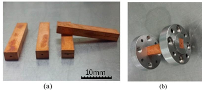
**Figure 11.** (a) The complete electromagnetic transmission channels of the WR2.8 waveguide after secondary machining. (b) The WR2.8 waveguide with flanges.
