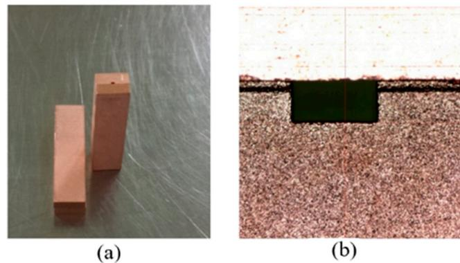
**Figure 10.** (a) Complete copper terahertz straight waveguide structures consisting of a channel block and a cover after bonding. (b) Cross-section of the waveguide structure.
