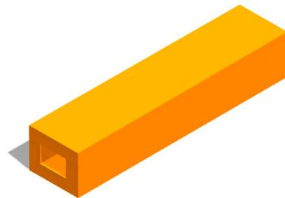
**Figure 3.** A complete electromagnetic transmission channel of a WR2.8 waveguide, consisting of a channel block and a copper plate cover.
