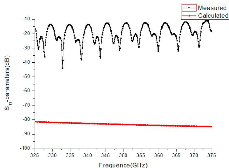
**Figure 16.** The experimentally measured  $S_{11}$  and calculated  $S_{11}$  parameters of the WR2.8 waveguide.
