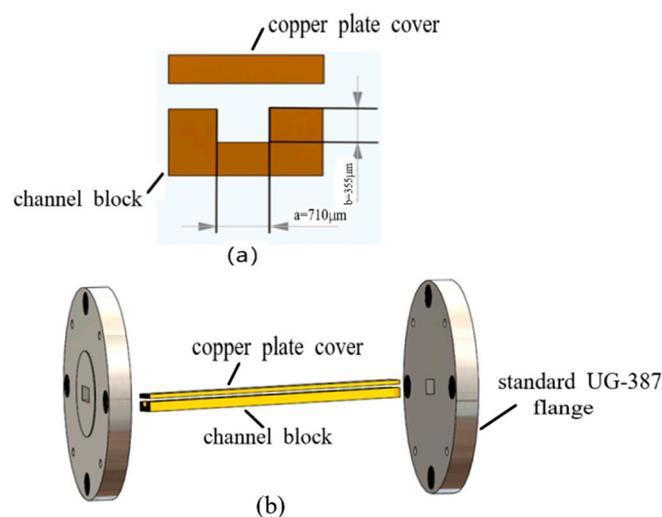
**Figure 1.** (a) A cross-sectional dimension of a WR2.8 rectangular waveguide:  $a = 710 \mu\text{m}$  and  $b = 355 \mu\text{m}$ . (b) A WR2.8 waveguide is composed of three parts: a channel block, a copper plate cover and standard UG-387 flanges.
