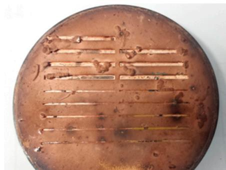
**Figure 8.** Optical microscope photograph of of the sample with 18 channels after SU-8 removal: 8 channels above for WR2.8, and 10 channels below for WR1.5.
