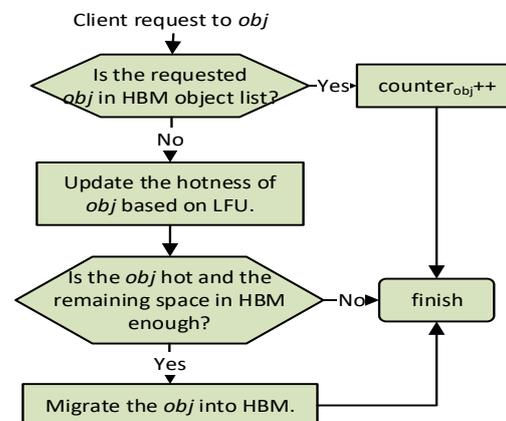
**Figure 3.** The migration workflow of HBM Migr-in from DRAM to HBM.
