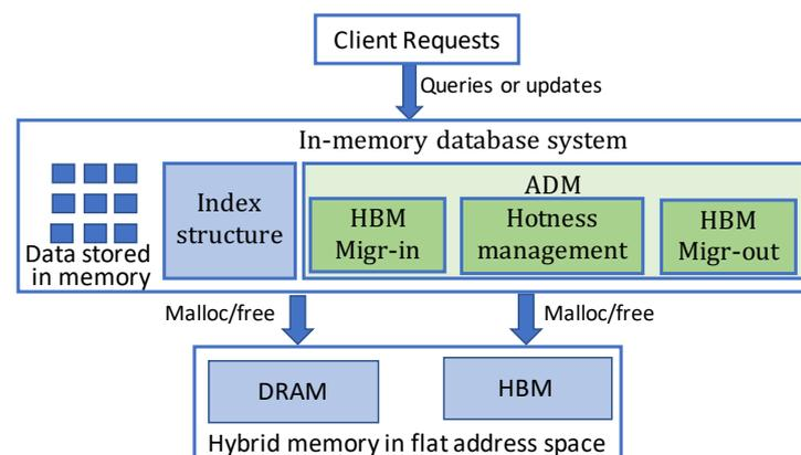
**Figure 2.** Overview of the proposed ADM method. ADM contains three components and is integrated to the Redis in-memory database.
