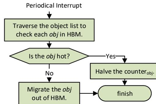
**Figure 4.** The migration workflow of HBM Migr-out from HBM to DRAM.
