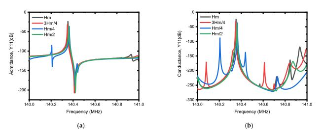
**Figure 11.** Illustration of simulated electrical responses using different patch depths (i.e.,  $H_m/4$ ,  $H_m/2$ ,  $3H_m/4$ , and  $H_m$ ). The patch depth ( $L_{patch}$ ) of  $W_e/3$  and the patch metal of tungsten (W) are used for the simulation. (a) Admittance, Y11 (dB), and (b) conductance, G (dB).
