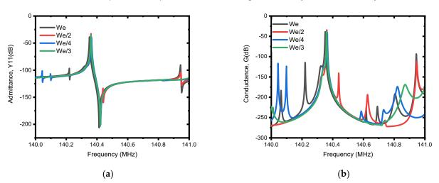
Figure 10. Illustration of simulated electrical responses using different patch lengths (i.e.,  $W_e/4$ ,  $W_e/3$ ,  $W_e/2$  and  $W_e$ ). The patch depth ( $H_{patch}$ ) of  $H_m/2$  and patch metal of tungsten (W) is used for the simulation. (a) Admittance, Y11 (dB), and (b) conductance, G (dB).
