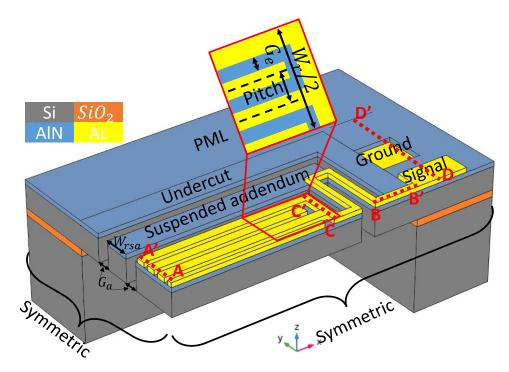
**Figure 3.** A mockup 3D view of a quarter plate resonator with an energy-preserving suspended addendum frame.
