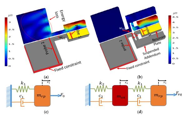
**Figure 1.** Illustration of: (a) Quarter plate conventional resonator used for the transmission test model along with its fundamental vibration mode shape at 140.32 MHz. (b) Quarter plate view of EPF resonator used for transmission test along with its fundamental vibration mode shape at 140.32 MHz. (c) Schematic view of a mass-spring-damper model used for the conventional MEMS resonator. (d) Schematic view of a mass-spring-damper model for a resonator with energy-preserving frames (EPF).
