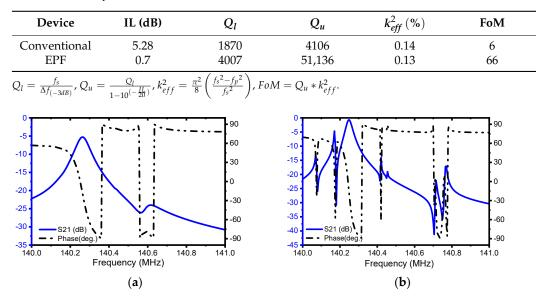
**Figure 7.** Illustration of the simulated S-parameter, S21 (dB) and phase (deg.) response of (**a**) the conventional resonator and (**b**) EPF resonator.
