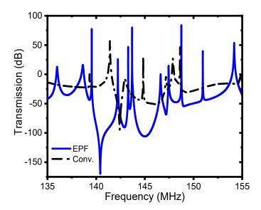
**Figure 2.** Transmission (dB) spectrum of the conventional and EPF resonators in the frequency range of 135 MHz to 155 MHz.
