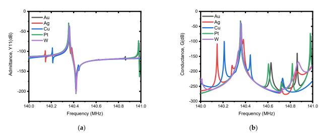
Figure 9. Illustration of simulated electrical responses with different patch metals (i.e., Au, Ag, Cu, Pt, and W). A patch length ( $L_{patch}$ ) of  $W_e/3$  and a patch depth ( $H_{patch}$ ) of  $H_2/m$  were used for the simulation. (a) Admittance, Y11 (dB), and (b) conductance, G(dB).
