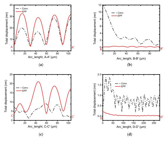
**Figure 5.** Illustration of the total displacement fields ( $\mu$ m) in the 7th-order width extension modes of the conventional and EPF resonators across the lines (**a**) A–A', (**b**) B–B', (**c**) C–C', and (**d**) D–D'. The significantly higher vibration at the tether and the anchoring boundary of the conventional resonator compared to the others revealed the higher anchor loss endured by it.
