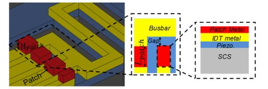
**Figure 8.** Schematic showing the proposed layout of metal patches on the edges of electrodes (inset: top view and side view of the selected regions at the edge of the IDT electrodes).
