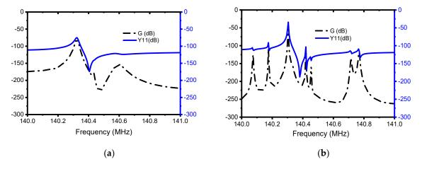
**Figure 6.** Illustration of the simulated admittance, Y11 (dB), and conductance, G (dB), response of the: (**a**) conventional resonator and (**b**) EPF resonator.
