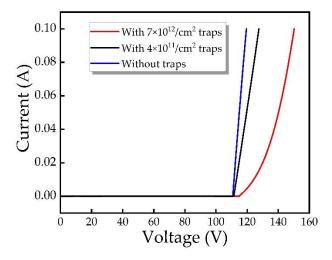
Figure 14. Reverse IV curve of DDR IMPATT with and without interface traps.
