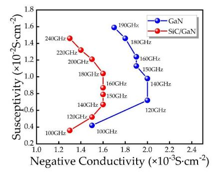
Figure 10. Admittance characteristics of IMPATT devices with different structures.
