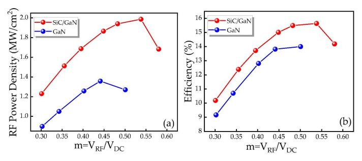
Figure 13. (a) RF power and (b) efficiency as a function of the voltage modulation factor *m* at 150 GHz.
