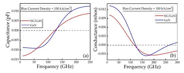
Figure 6. (a) Capacitance and (b) conductance as a function of frequency for different IMPATT diodes.
