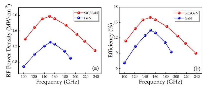
Figure 11. The relationship between (a) RF power, (b) efficiency and frequency of different IMPATT diodes.
