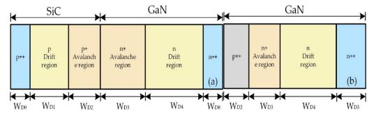
Figure 1. (a) The DDR IMPATT diode and (b) SDR IMPATT diode structure comparison diagram.
