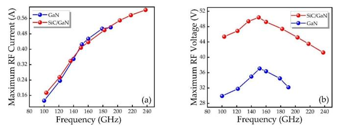
Figure 8. (a) RF current and (b) RF voltage as a function of frequency of different IMPATT diodes.
