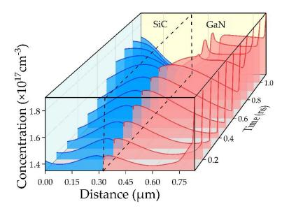
**Figure 15.** Concentration distribution of holes and electrons in the DDR IMPATT at a fixed time interval of one tenth period at 150 GHz.
