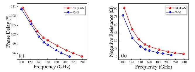
Figure 9. The relationship between (a) phase delay, (b) negative resistance and frequency of different IMPATT diodes.
