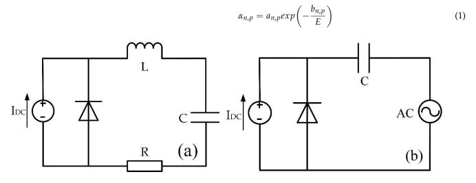
Figure 2. (a) The free-running and (b) voltage-driven oscillation circuit diagram.
