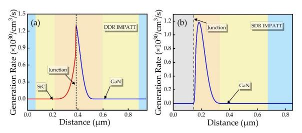
Figure 5. Impact-ionization generation rate as a function of distance. (a) SiC/GaN DDR, (b) GaN SDR.
