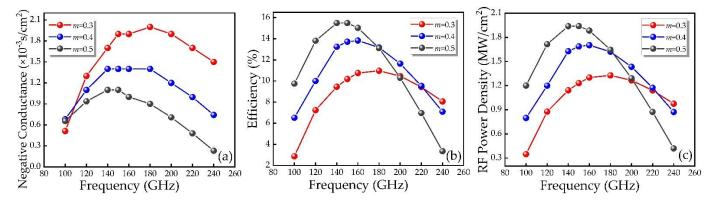
**Figure 12.** (a) Negative conductance, (b) efficiency and (c) RF power as a function of the frequency of the SiC/GaN DDR IMPATT under different voltage modulation factors *m*.
