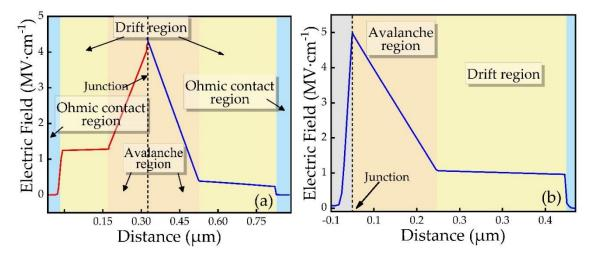
Figure 4. Electric field of (a) DDR IMPATT and (b) SDR IMPATT as a function of distance.
