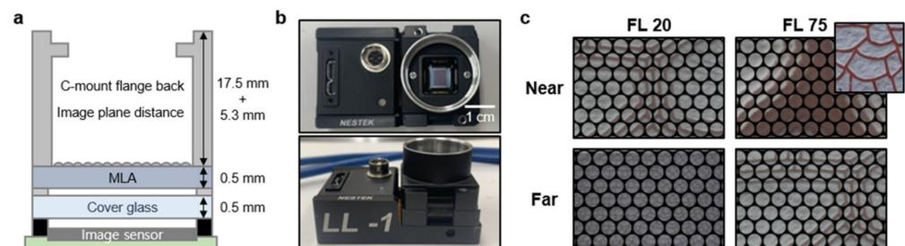
**Figure 3.** (a) Schematic of optical alignment module for VF-LFC. (b) Photographs of the assembled module for VF-LFC (c) Photographs of light field image captured by VF-LFC with focal length FL 20 mm (left), and FL 75 mm (right), inset: original texture image.
