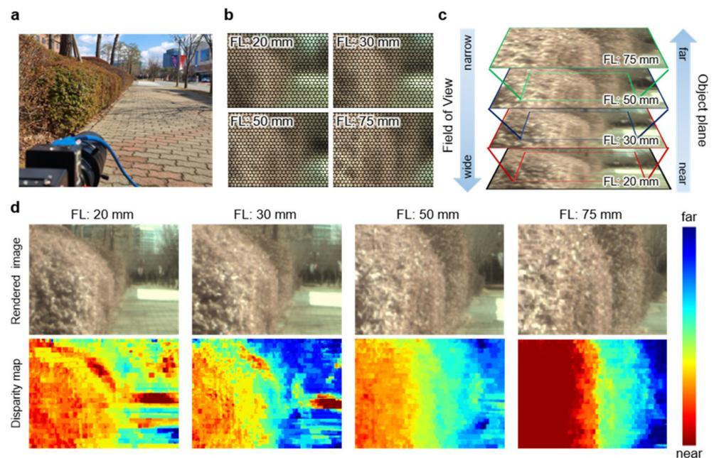
**Figure 5.** (a) Photograph of outdoor measurement setup of VF-LFC. (b) Microimages from VF-LFC at four different focal lengths. (c) Photographs indicating the field of view difference and object distance for each focal length. (d) Photographs after image rendering (top row) and disparity maps according to each focal length captured by a VF-LFC (bottom row).
