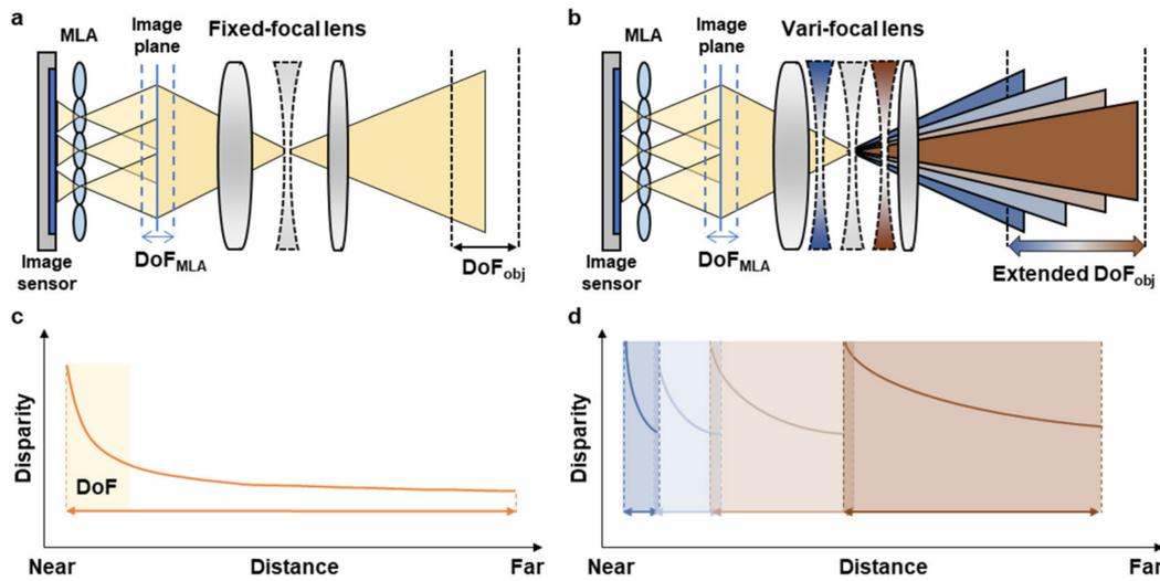
**Figure 1.** (a,b) Schematic of conventional light field camera (a) and proposed light field camera with a vari-focal lens (b). (c,d) Relationship between disparity and object distance. (c) The disparity of the conventional light field camera decreases and converges. (d) By controlling the focal length before the disparity converges, the proposed VF-LFC provides an extremely extended DoF.
