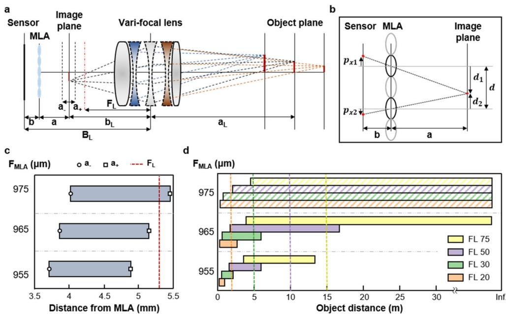
**Figure 2.** (a) Schematic of the VF-LFC system with main design parameters. (b) Schematic of the optical path through the MLA between the image sensor and the image plane of the main lens. (c) The image side DoF,  $a_+$  and  $a_-$ , are calculated from the thin lens equation for a focal length of MLA. (d) The object side DoF for each focal length of a vari-focal lens according to the MLA focal length, the dotted lines are the boundaries between measurement regions of each focal length.
