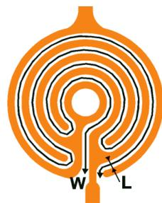
**Figure 2.** Structure of the comb-shaped sensing electrodes.
