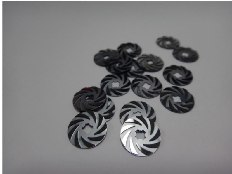
**Figure 3.** Fabricated MEMS turbine rotor.
