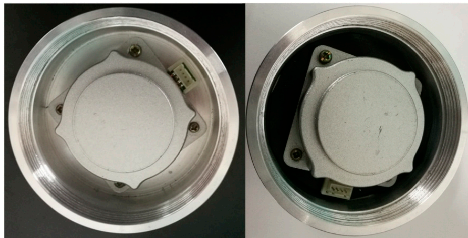
Figure 13. Ultrasonic motor with (right) and without (left) the protection of rubber.
