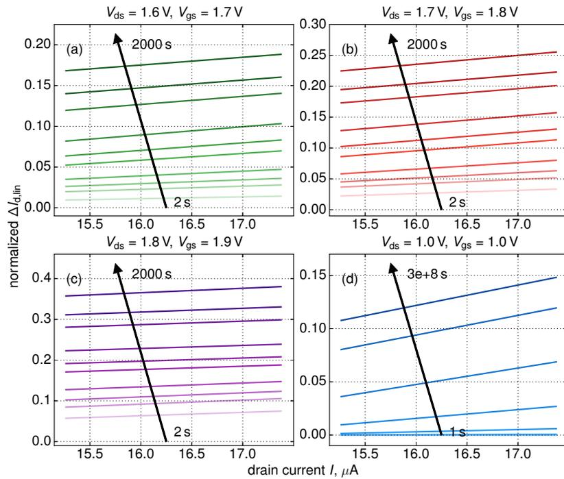
**Figure 7.**  $\Delta I_{d,lin}(I_{d,lin}^{(0)})$  dependencies for all stress time steps and four combinations of  $V_{ds}$ ,  $V_{gs}$ . As opposed to Figure 6 showing additionally normalized  $\Delta I_{d,lin}(t) / \langle \Delta I_{d,lin} \rangle$  traces this figure depicts relative changes of the linear drain current, i.e.,  $\Delta I_{d,lin}(t) = |I_{d,lin}(t) - I_{d,lin}(0)| / I_{d,lin}(0)$ .
