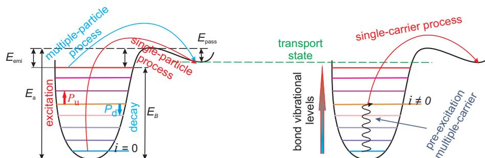
**Figure 2.** Single- and multiple-carrier mechanisms of Si-H bond rupture (left panel) and their superposition (right panel).
