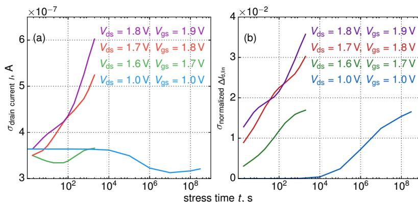
**Figure 5.** The standard deviations of the linear drain  $I_{d,lin}$  (a) and the relative linear drain current change  $\Delta I_{d,lin}$  (b) as functions of stress time  $t$ .
