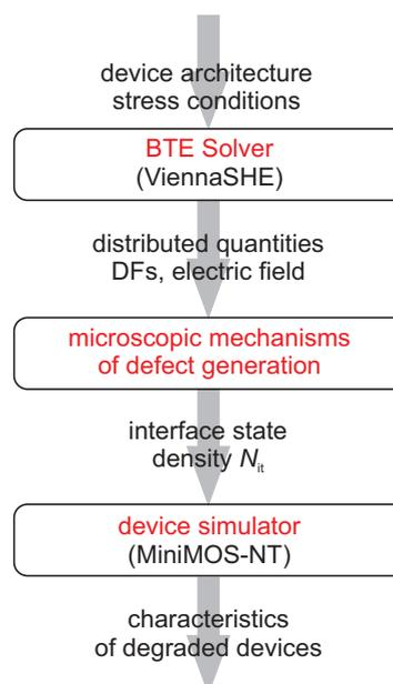
**Figure 1.** The schematic representation of our modeling framework which covers and links three main sub-tasks of the problem of hot-carrier degradation: modeling of carrier transport, modeling of the defect generation rates, and simulations of the degraded devices.
