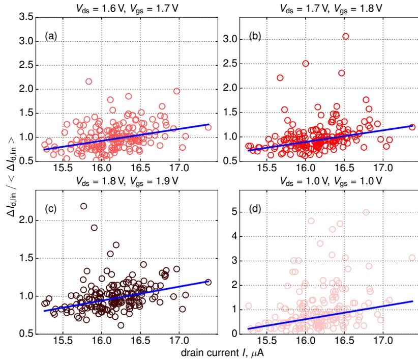
**Figure 6.**  $\Delta I_{d,\text{lin}}(t) / \langle \Delta I_{d,\text{lin}} \rangle$  values plotted vs.  $I_{d,\text{lin}}^{(0)}$  currents. Data for all four stress conditions and stress time of 2 s are shown. Note that  $\Delta I_{d,\text{lin}}$  changes are normalized to the mean linear drain current change  $\langle \Delta I_{d,\text{lin}} \rangle$ .
