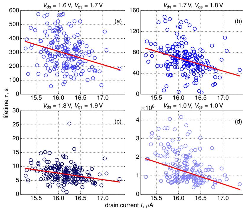
**Figure 9.** Extracted dependencies of device lifetime  $\tau$  on  $I_{d,lin}^{(0)}$  for all stress conditions. To evaluate device lifetime values we used a  $\Delta I_{d,lin} = 0.1$  criterion.
