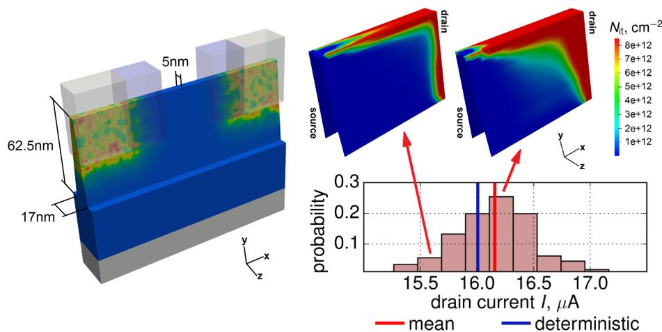
**Figure 3.** A sketch of the n-FinFET with random dopants (left), the distribution of the time-0 linear drain currents  $I_{d,lin}^{(0)}$  and  $N_{it}$  densities obtained at  $V_{ds} = 1.8 \text{ V}$ ,  $V_{gs} = 1.9 \text{ V}$  and  $t = 200 \text{ s}$  for two different  $I_{d,lin}^{(0)}$  values (right).
