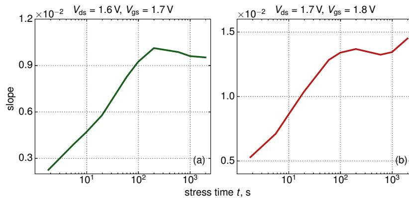
**Figure 8.** The slope of the  $\Delta I_{d,lin}(I_{d,lin}^{(0)})$  dependency as a function of stress time  $t$  for  $V_{ds} = 1.6$  V,  $V_{gs} = 1.7$  V and  $V_{ds} = 1.7$  V,  $V_{gs} = 1.8$  V.
