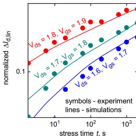
**Figure 4.** Experimental and simulation  $\Delta I_{d,lin}(t)$  degradation traces are in good agreement for all three stress conditions. The data are from [36].
