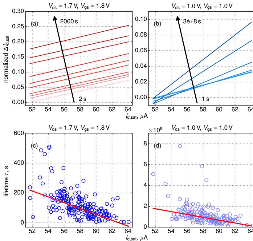
**Figure 10.** Extracted  $\Delta I_{d,sat}(I_{d,sat}^{(0)})$  dependencies for all stress time steps (a,b) and device lifetime obtained using  $\Delta I_{d,sat}$  traces (c,d).
