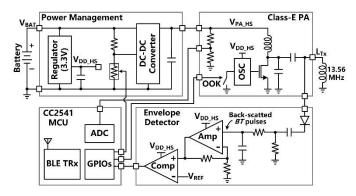
Figure 5. Block diagram of the headstage.
