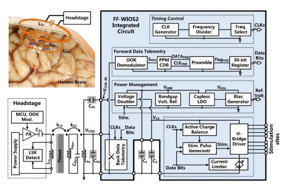
Figure 2. Block diagram of the FF-WIOS2 system-on-chip (SoC) architecture.
