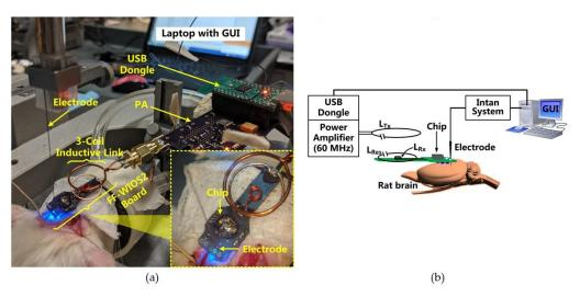
Figure 6. (a) In vivo experimental setup with its (b) block diagram.
