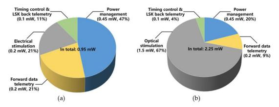
**Figure 12.** Power consumption of each block in the FF-WIOS2 device when applying (**a**) electrical stimulation and (**b**) optical stimulation.
