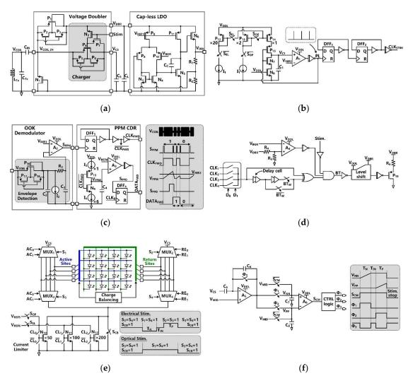
**Figure 3.** Schematic diagram of (**a**) the voltage doubler with built-in charger and the cap-less LDO, (**b**) the clock generator for the timing of stimulation and charging functions, (**c**) the OOK demodulator and PPM-CDR in forward data telemetry, (**d**) the LSK back telemetry, (**e**) the stimulation driver in H-bridge configuration, and (**f**) the active charge balancing (CB) circuit.
