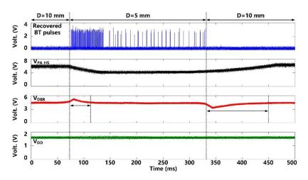
**Figure 11.** Measured waveforms under CLPC operation, when moving the headstage to change the distance between  $L_{\text{Tx}}$  and  $L_{\text{Res}}$ , *D*.
