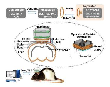
**Figure 1.** Conceptual view of the system setup for operating multiple mm-sized free-floating wirelessly-powered implantable opto-electro stimulation (FF-WIOS2) devices, distributed on a freely moving rat brain.
