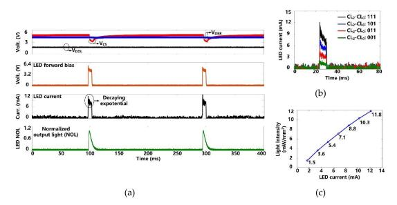
**Figure 9.** (a) Measured optical stimulation waveforms. (b) Measured  $\mu$ LED current at different stimulation current settings. (c) Measured light intensity as a function of the  $\mu$ LED current.
