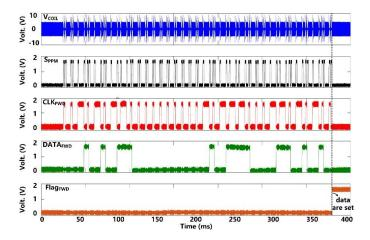
Figure 8. Measured results of forward data telemetry.
