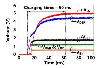
Figure 7. Transient waveforms of the power management block at starting up.
