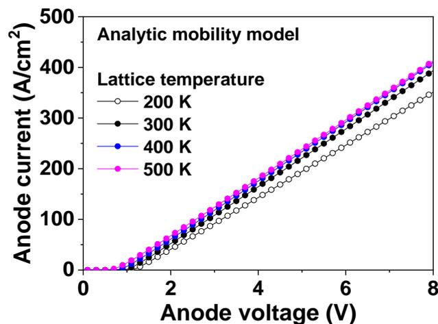
**Figure S1.** Forward current–voltage (I–V) characteristics of the p-type diamond pseudo-vertical Schottky barrier diode (SBD) simulated using the analytic mobility model at 200, 300, 400, and 500 K. The metal work function and hole saturation velocity were 5.65 eV and  $2.7 \times 10^7$  cm/s respectively.
