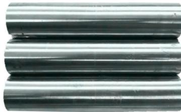
**Figure 8.** Titanium-alloy tubes.
