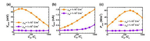
**Figure 6.** (a) Simulated osmotic voltage, (b) osmotic current, and (c) maximum osmotic power density as a function of the concentration gradient for the two levels of space charge densities. The lower salt concentration is fixed at 1 mM.
