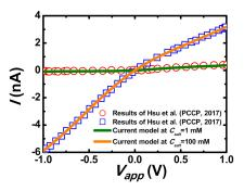
**Figure 2.** Code validation by comparing the results from the current model (solid curves) with the previous results of Hsu et al. [57], who modeled the current-voltage curves of a polyelectrolyte (PE)-modified nanopore at the two levels of KCl concentrations.
