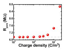
**Figure 5.** Resistance ( $R_{pore}$ ) of the considered mesopore system as a function of  $\rho_{PE}$  in a 1000 mM/1 mM salinity gradient. The dashed curve represents the result from the bare solid-state mesopore system.
