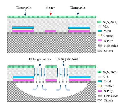
**Figure 3.** Fabrication steps of proposed sensor using a complementary metal-oxide-semiconductor (CMOS)-compatible process.
