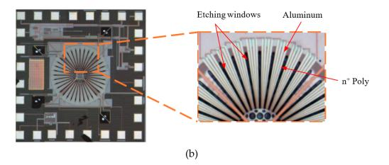
Figure 2. (a) Schematic drawing of the thermopile structure; (b) Photography of chip after fabrication.
