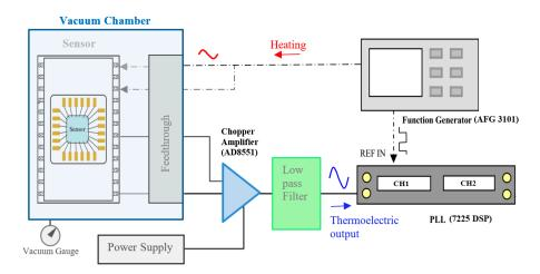
Figure 4. Setup of vacuum chamber and signal processing architecture.
