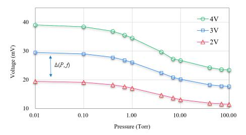
Figure 11. Output voltage versus pressure under various bias voltages applied to heater at 10 Hz.
