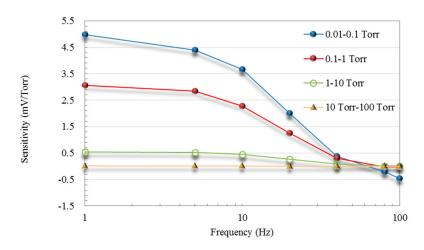
Figure 8. Sensitivity vs. frequency across various ranges of vacuum pressure.
