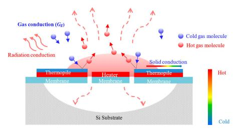
Figure 1. Sensing scheme of proposed thermoelectric-type sensor.
