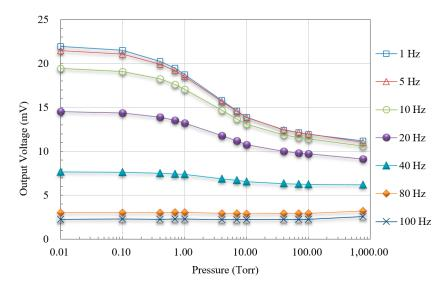
Figure 6. Output voltage versus pressure under different modulation frequencies.
