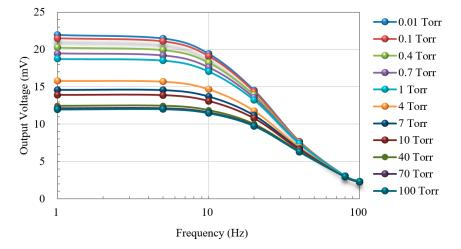
Figure 5. Output voltage versus frequency of input bias voltage applied to the heater.
