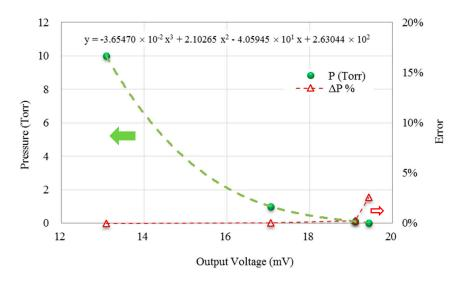
Figure 9. Calibration and error analysis of vacuum measurement at 10 Hz.
