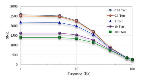
Figure 10. Signal-to-noise ratio (SNR) versus frequency for different pressures.
