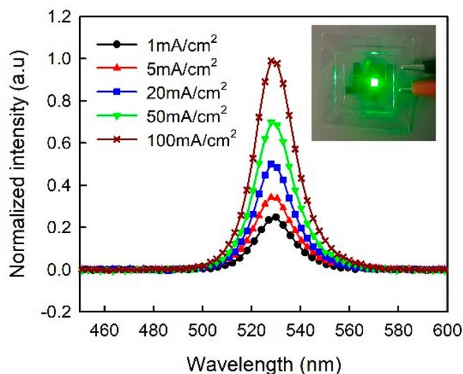
**Figure 7.** EL spectra of the PeLED devices with a three-step spin-coated emitter and a PEDOT:PSS/MoO<sub>3</sub>-ammonia (1:0.02) composite HTL at different current densities. The inset is a luminescence image of the device at 50 mA/cm<sup>2</sup>.
