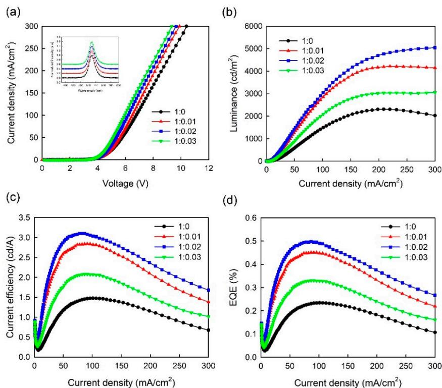
**Figure 6.** (a) J-V, (b) L-J, (c) CE-J, (d) EQE-J curves of PeLEDs with a three-step spin-coated emitter and a PEDOT:PSS/MoO<sub>3</sub>-ammonia (1:0, 1:0.01, 1:0.02, 1:0.03) composite HTL (device T1, T2, T3, T4). The inset is normalized EL spectra of the PeLED devices at 20 mA/cm<sup>2</sup>, which were shifted vertically for clarity.
