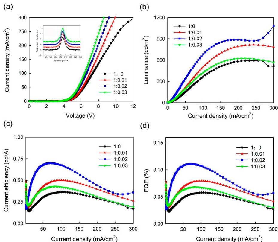
**Figure 5.** (a) J-V, (b) L-J, (c) CE-J, (d) EQE-J curves of PeLEDs with a one-step spin-coated emitter and a PEDOT:PSS/MoO<sub>3</sub>-ammonia (1:0, 1:0.01, 1:0.02, 1:0.03) composite HTL (device S1, S2, S3, S4). The inset is normalized EL spectra of the PeLED devices at 20 mA/cm<sup>2</sup>, which were shifted vertically for clarity.
