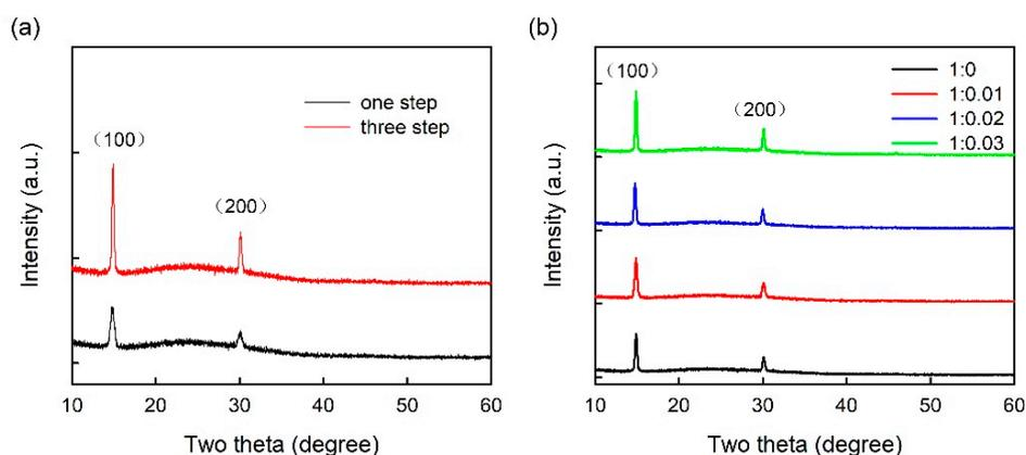
**Figure 3.** XRD patterns of (a) one-step and three-step coated  $\text{CH}_3\text{NH}_3\text{PbBr}_3$  films on the pure PEDOT:PSS film, (b) three-step coated  $\text{CH}_3\text{NH}_3\text{PbBr}_3$  films on the pure PEDOT:PSS film and PEDOT:PSS/ $\text{MoO}_3$ -ammonia composite HTLs with different  $\text{MoO}_3$  ratios. The XRD patterns were shifted vertically for clarity.
