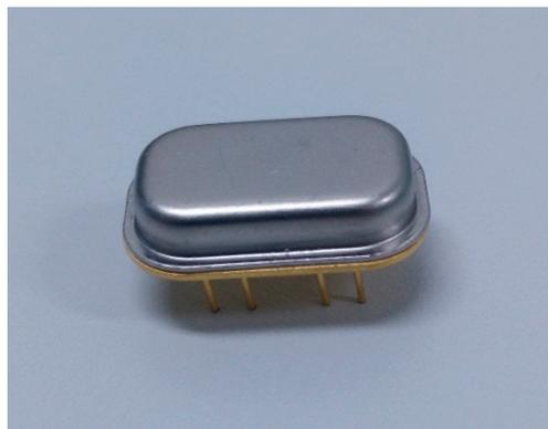
**Figure 10.** Metal vacuum packaging for the AlN MEMS gyroscope.
