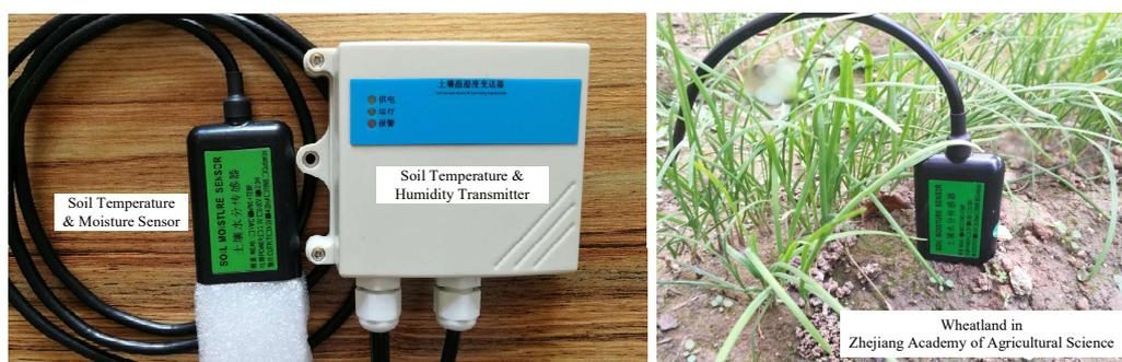
Figure 1. Temperature and moisture sensor deployed in the wheatland.
