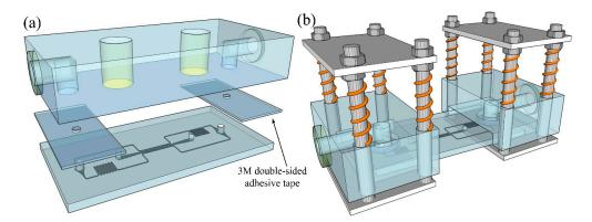
Figure 3. Schematic of the assembled RSUIM with the generic organ-on-a-chip module.(a) Pasting-based RSUIM assembly with 3M double-sided transparent adhesive tape.(b) Clamping-based RSUIM assembly by the clamping force from springs.
