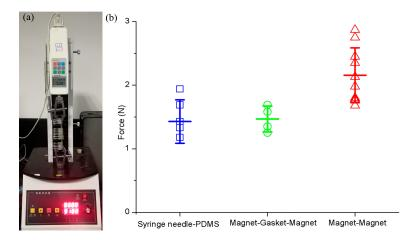
Figure 5. Characterization on attraction strength among different connection modes. (a) Tensile test machine. (b) Characterization results.
