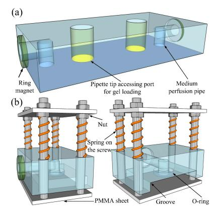
**Figure 1.** Schematic of two different types of reusable standardized universal interface module (RSUIM) design. (a) Pasting-based RSUIM design, (b) clamping-based RSUIM design.
