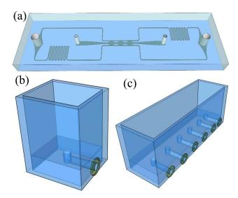
**Figure 2.** Schematic of the generic vascularized organ-on-a-chip and medium reservoir modules design. (a) Coupling design of the microfluidic chip with two medium perfusion ports and two gel loading ports. (b) Medium reservoir module with only one medium access port. (c) Medium reservoir module with six medium access ports.
