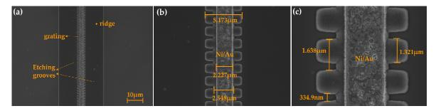
**Figure 6.** SEM images of a top view of the fabricated DFB laser diodes with 20th order sidewall gratings. (a) An overall view of the DFB LD with double etching grooves; (b) a low power and (c) a high power perspective of the ridge waveguide and the sidewall gratings along it.
