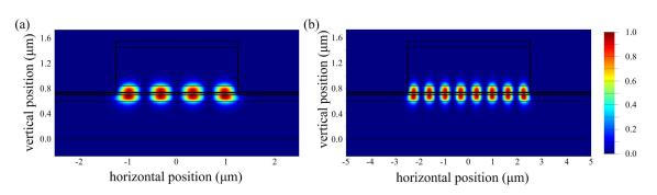
**Figure 1.** Optical field profiles for ridge widths of (a) 2.5  $\mu$ m and (b) 5  $\mu$ m.
