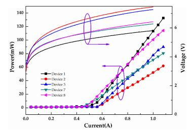
**Figure 8.** Light output power–current–voltage characteristics of Devices 1, 2, 3, 7, and 8 operated in pulsed mode with a 1  $\mu$ s pulse width and a 10 kHz repetition rate.
