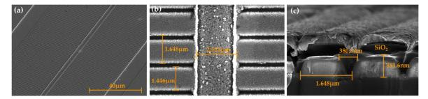
**Figure 4.** Scanning electron microscope (SEM) images of (a) an oblique view of the fabricated DFB laser diodes with surface gratings, (b) a top vision of the 20th order surface gratings alongside a metal stripe, and (c) a sectional structure of the surface gratings perpendicular to the facet of LDs.
