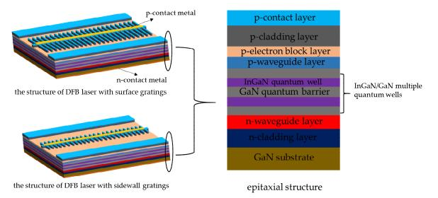
**Figure 3.** The structures of processed distributed feedback laser diodes (DFB-LDs) with surface gratings and sidewall gratings, as well as the diagrammatic drawing of the cross profile of the gallium nitride (GaN)-based epitaxial wafer.
