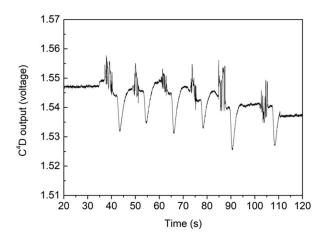
Figure S2. Response to the injection of 0.1  $\mu$ M KCl solution. The flow velocity is 3  $\mu$ L/min of DI water, and the injection volume of sample is 1 nL.
