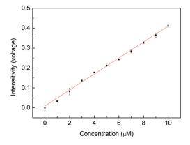
**Figure S1.** The C<sup>4</sup>D detection of different concentrations of the potassium chloride solution from 1 to 10  $\mu$ M (R2 = 0.9885).
