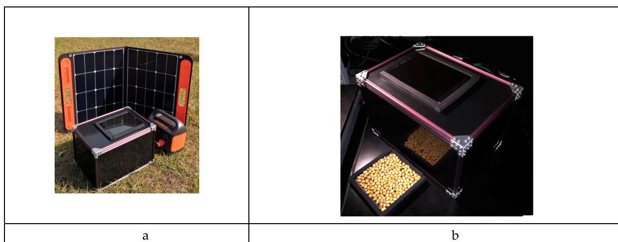
Figure S2. The prototype portable aflatoxin contamination detection device employs a tablet for fluorescence imaging of maize samples. a . Device with solar power, b . Prototype detection device with sample tray.
