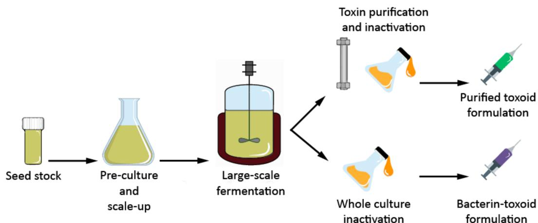
**Figure 2.** The production steps in a typical clostridial vaccine production process.
