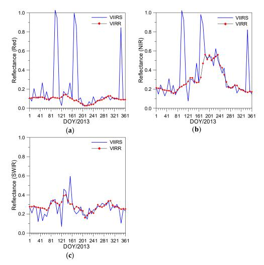
**Figure 2.** Temporal profiles of VIIRS surface reflectance and reconstructed surface reflectance using the VIRR method for the center pixel of the AGRO site in 2013. (a) Surface reflectance in the red band; (b) surface reflectance in the NIR band; (c) surface reflectance in the SWIR band.
