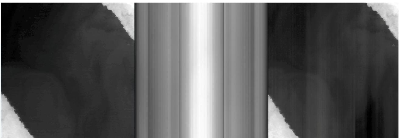
**Figure 9.** Real TIRS image of the Red Sea (**left**) and DIRSIG-generated simulated image (**right**). Similar banding artifacts observed in the actual TIRS scene are reproduced in the DIRSIG scene.
