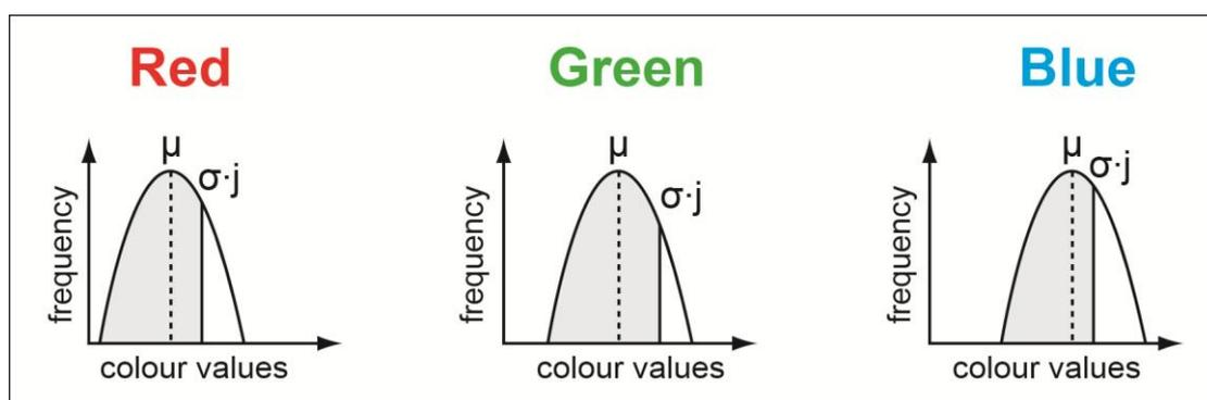
Several layers are calculated within a defined range and step size of  $j$ . A fuzzy segment boundary is created by summing up the resulting layers for each value of parameter  $j$ . The summed up layers
