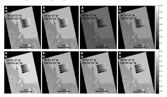
The band shapes of all detectors within a spectral band were grouped into classes. The mean band shape of the two most different classes were provided by NASA Goddard to apply to the synthetic scene. To determine the effect of the two different band shapes within a TIRS channel, each class mean band shape was applied separately to every detector on the DIRSIG scene. In addition, each band
