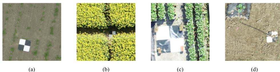
**Figure 4.** Examples of  $512 \times 512$ -pixel tiles, (a) a perfectly visible GCP, (b) GCP partially covered by the crop, (c) GCP reflecting sunlight, (d) GCP covered by sand.
