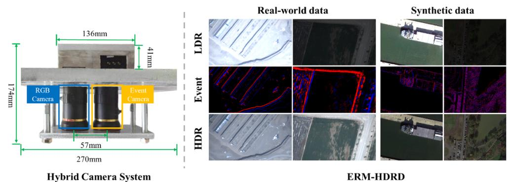
**Figure 5.** The details of our proposed datasets. (Left): the hardware implementation of our hybrid camera system. (Right): samples from our proposed ERS-HDRD dataset, composed of both real-world and synthetic data.
