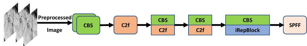
**Figure 8.** Structure of the improved darknet.
