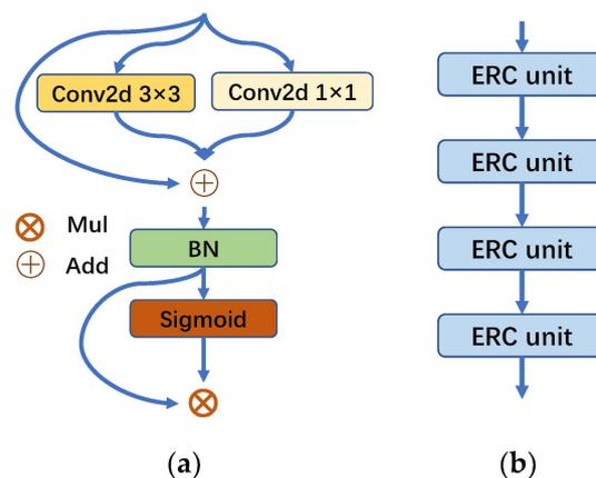
**Figure 9.** Structure of the improved neck and ERC blocks: (a) ERC unit and (b) ERC block.
