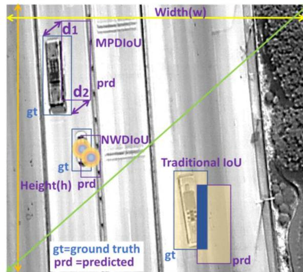
**Figure 11.** Schematic diagram of traditional IoU, NWDIoU, and MPDIoU.
