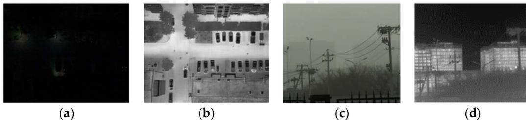
**Figure 1.** Advantages of infrared images compared with visual images. (a) Visual image at night, (b) infrared image at night, (c) visual image in fog, and (d) infrared image in fog.
