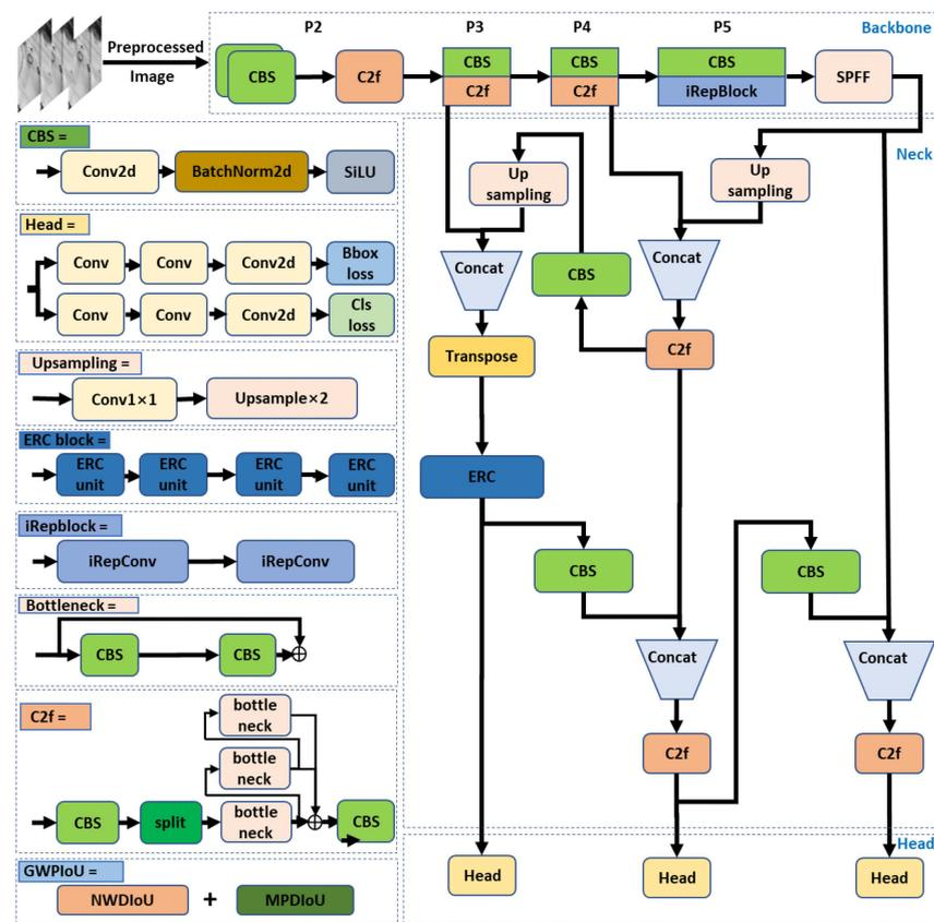
Figure 6. Overall ERGWnet structure.
