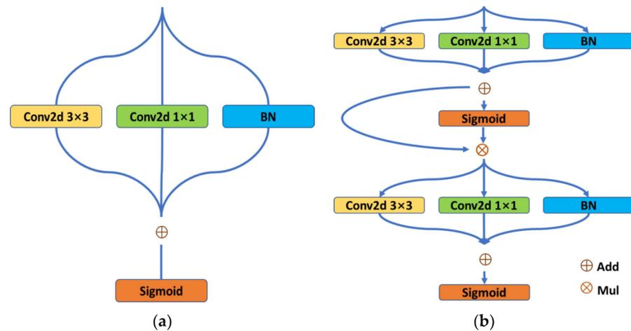
Figure 7. Improved RepConv and Repblock: (a) improved RepConv and (b) improved Repblock.
