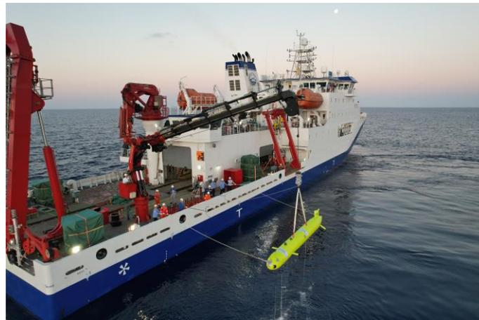
**Figure 4.** Situation at the site of the AUV deployment operation.
