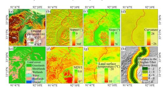
**Figure 3.** Environmental factors extracted in the study area: (a) Ground elevation; (b) Aspect; (c) Slope; (d) Curvature; (e) Land cover; (f) NDVI; (g) Land surface temperature; (h) Distance to the Qinghai–Tibet Highway.
