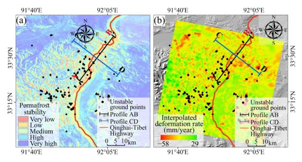
**Figure 11.** Permafrost stability mapping in the study area: (a) Results of the permafrost stability mapping with the trained random forest model; (b) Ground deformation rate obtained by the Kriging interpolation of initial InSAR analysis (Note: Profiles AB and CD are delineated to compare the two permafrost stability results).
