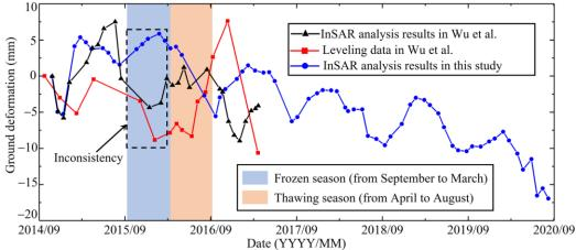
**Figure 15.** Verifications of the time-series InSAR analysis results with the leveling data and InSAR analysis results obtained by Wu et al. [39] (Reprinted with permission from ref. [39]. Copyright 2018 Copyright Sciences in Cold and Arid Regions).
