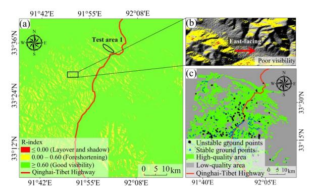
**Figure 10.** Screening analysis of the InSAR analysis results of ground deformation in the study area: (a) Geometric distortion analysis results; (b) A detailed survey of the geometric distortions on an east-facing slope; (c) Zonation of the high-quality and low-quality areas.
