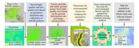
**Figure 2.** Principle and implementation procedures of the integrated method for permafrost stability mapping.
