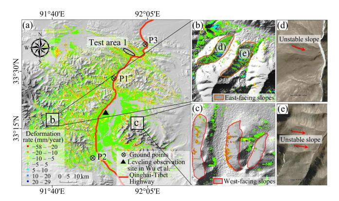
**Figure 4.** InSAR analysis results of the ground deformation in the study area: (**a**) Vertical ground deformation rate from October 2014 to August 2020 [39]; (**b**) Ground deformation rate in east-facing slopes; (**c**) Ground deformation rate in west-facing slopes; (**d**,**e**) Google Earth images for east-facing slopes (Image from © Google Earth 2020).
