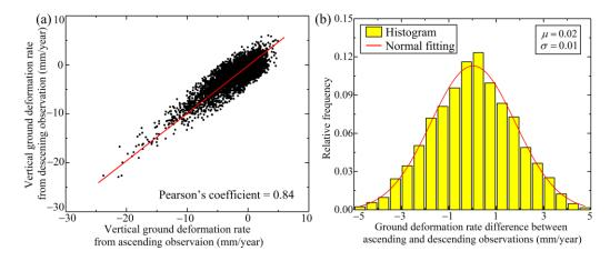
**Figure 18.** Comparison of the ground deformation rate obtained from ascending and descending SAR images: (a) Correlation analysis of the vertical ground deformation rates obtained from ascending and descending SAR images; (b) Distribution of the ground deformation rate differences between ascending and descending SAR images.
