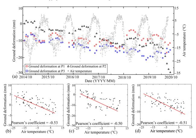
**Figure 16.** Relationships between the ground deformation and the air temperature: (**a**) Relationships between the ground deformation and the air temperature at points P1, P2, and P3; (**b**–**d**) Correlations between the ground deformation and the air temperature at points P1, P2, and P3.
