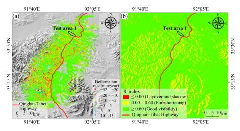
**Figure 17.** InSAR analysis results in the study area obtained from the ascending Sentinel-1 SAR images: (a) Vertical ground deformation rate from October 2014 to August 2020; (b) Geometric distortion analysis results.
