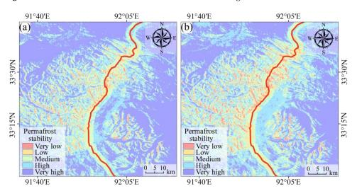
**Figure 13.** Permafrost stability mapping using different classification schemes: (**a**) Equal intervals; (**b**) Standard deviations.
