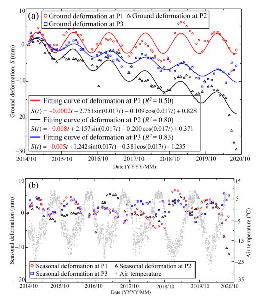
**Figure 5.** Fitting analysis of the ground deformation in the period from 2014 to 2020: (**a**) Fitting analysis between the ground deformation and the time; (**b**) Correlation analysis between the seasonal deformation and the air temperature (note: the air temperature is from the 2.0 m air temperature dataset from the European Centre for Medium-Range Weather Forecasting—Fifth-Generation Reanalysis (ECMWF ERA5)).
