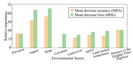
Figure 14. The relative importance of the environmental factors to the permafrost stability.
