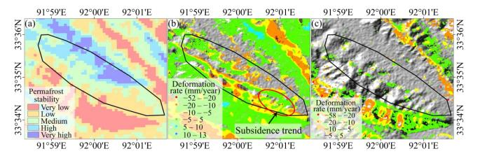
**Figure 19.** Comparisons between the permafrost stability mapping results in Test Area 1 obtained with the proposed method and the ground deformations obtained from the ascending SAR images: (a) Permafrost stability mapping results obtained with the proposed method; (b) Vertical ground deformation rates obtained from the ascending SAR images; (c) Vertical ground deformation rates obtained from the descending SAR images.
