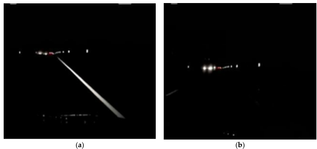
Figure 1. Comparison of lane markings in terms of visibility at night as a result of retroreflectivity performance: (a) adequate visibility and (b) inadequate visibility.
