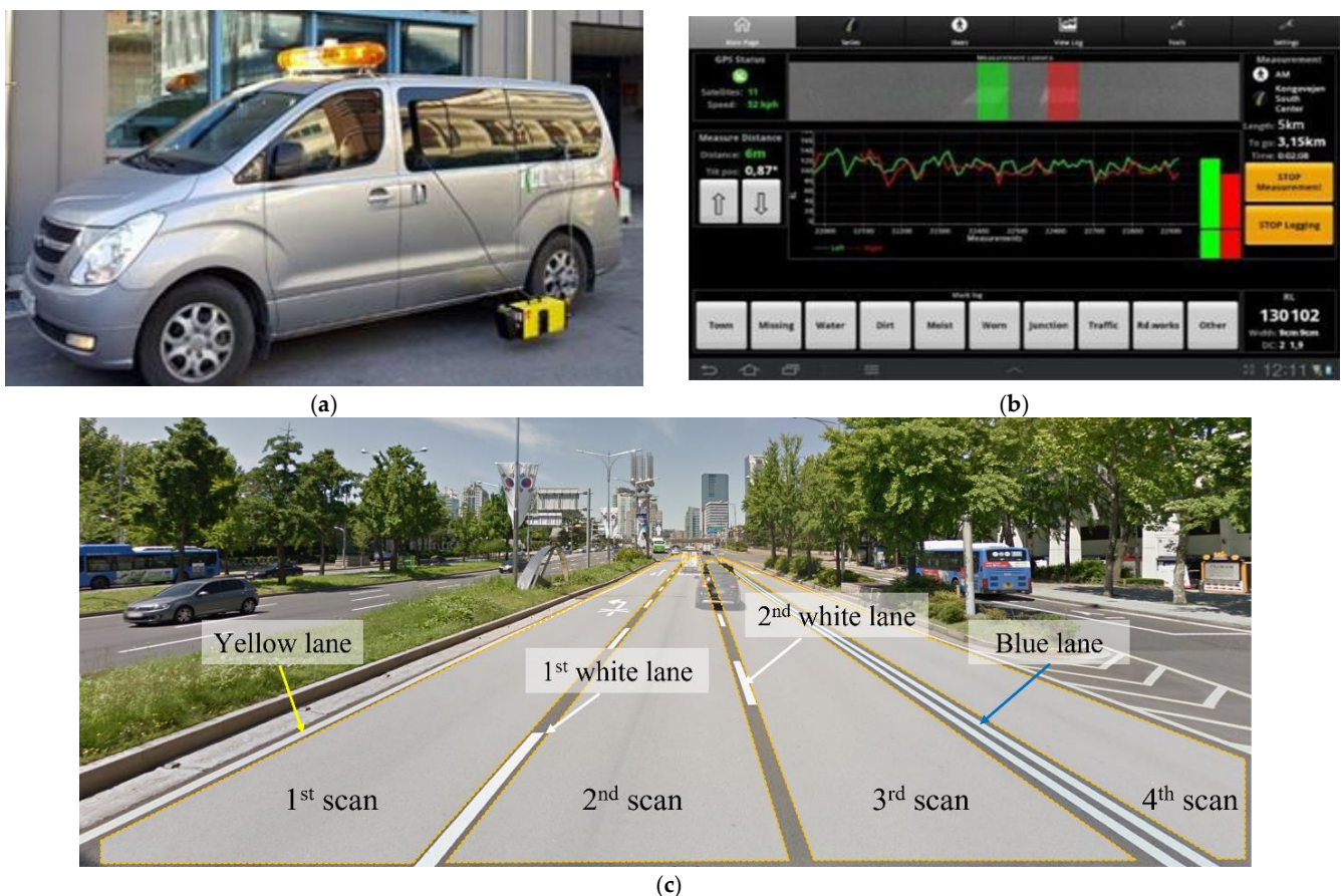
Figure 3. Overview of the retroreflectivity investigation program: (a) vehicle-mounted retroreflectometer, (b) real-time monitoring system, and (c) illustration of the scanning procedure for a four-lane road.
