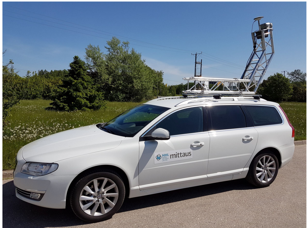
Figure 4. ROAMER R3 mobile laser scanning system installed on top of a truss structure mounted on a car.
