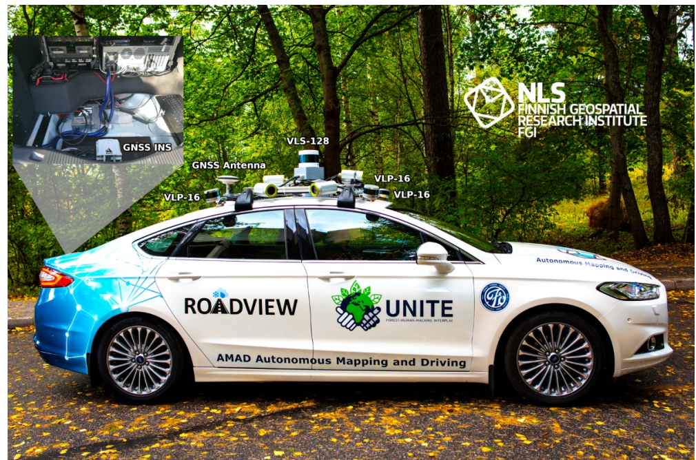
Figure 2. Photograph of the autonomous mapping and driving research platform, ARVO, which was used to record the autonomous perception data in this study. The inset shows the trunk of the ARVO car.
