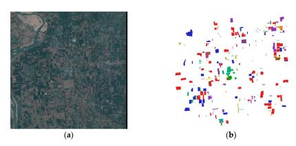
**Figure 2.** GF14 dataset false color images and ground truth: (a) three-band composite false color images (25, 11, 7); (b) ground truth.
