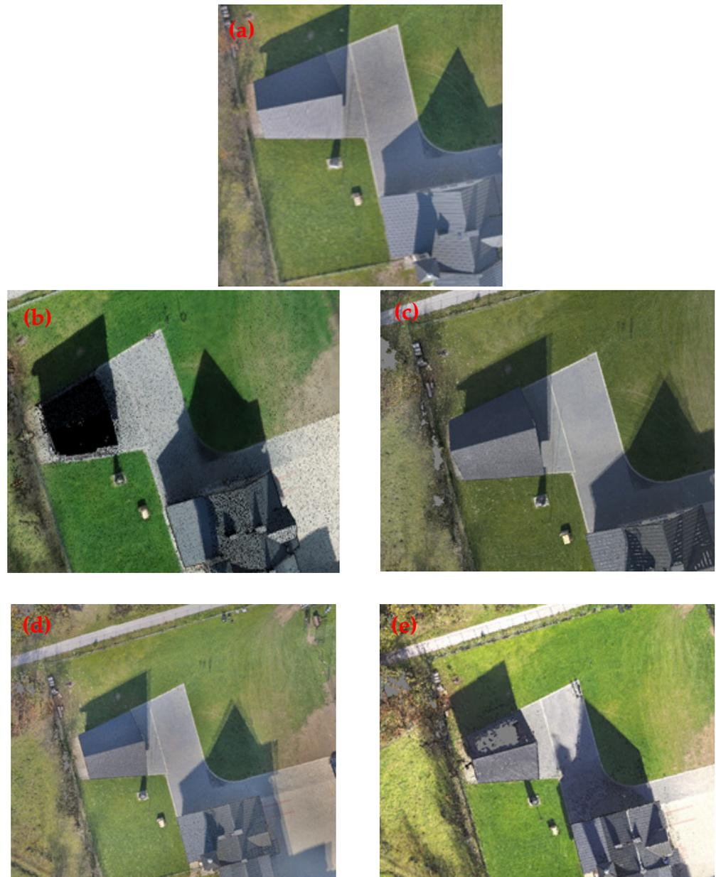
**Figure 9.** Lack of information for roof planes in point clouds example 3 (a) photos of roof planes (b) point cloud from L1 scanner, (c) point cloud from DNG files, P1 camera, (d) point cloud from TIF files, P1 camera, (e) point cloud from JPG files PSDK camera.
