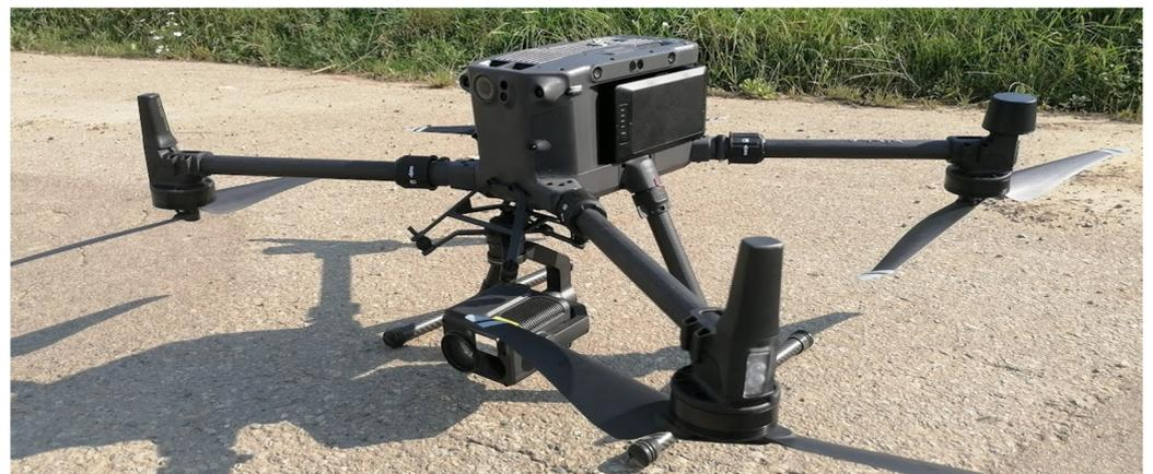
**Figure 2.** Measuring equipment: DJI Matrice 300 RTK with DJI Zenmuse L1 laser scanner.
