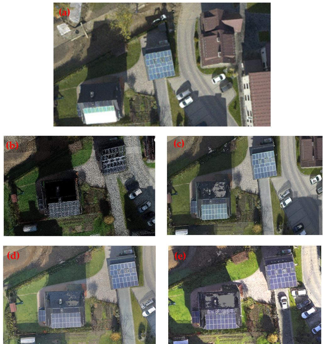
**Figure 8.** Missing information for roof planes in point clouds example 2 (a) photos of roof planes (b) point cloud from L1 scanner, (c) point cloud from DNG files, P1 camera, (d) point cloud from TIF files, P1 camera, (e) point cloud from JPG files PSDK camera.
