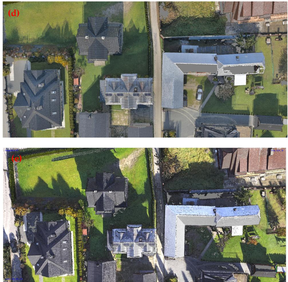
**Figure 7.** Missing information for roof planes in point clouds example 1 (a) photos of roof planes (b) point cloud from L1 scanner, (c) point cloud from DNG files, P1 camera, (d) point cloud from TIF files, P1 camera, (e) point cloud from JPG files PSDK camera.
