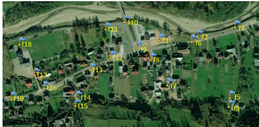
**Figure 5.** Distribution of ground control points in the surveyed area.
