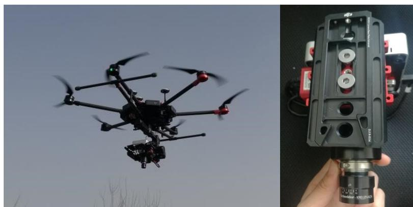
**Figure 2.** Resonon-Pika-L airborne imaging spectrometer.
