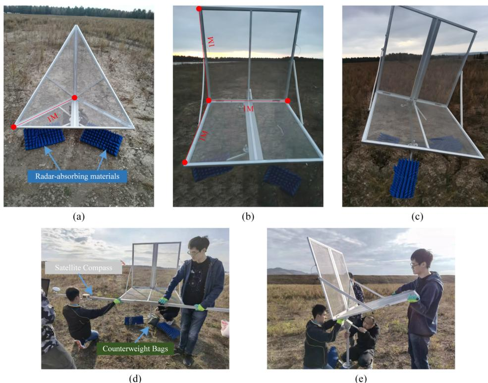
**Figure 5.** Ground-deployed CRs at Yudaokou Airport in September 2021: (a–c) trihedral CR, dihedral CR, and  $22.5^\circ$  rotated dihedral CR, respectively; (d,e) placement process and measuring equipment.
