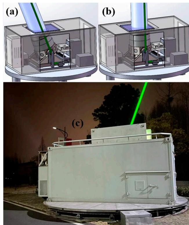
**Figure 1.** Active Rotating Tropospheric Stratospheric Doppler Wind Lidar. (a) Tilt detection mode. (b) Vertical detection mode. (c) Schematic diagram of detection work.
