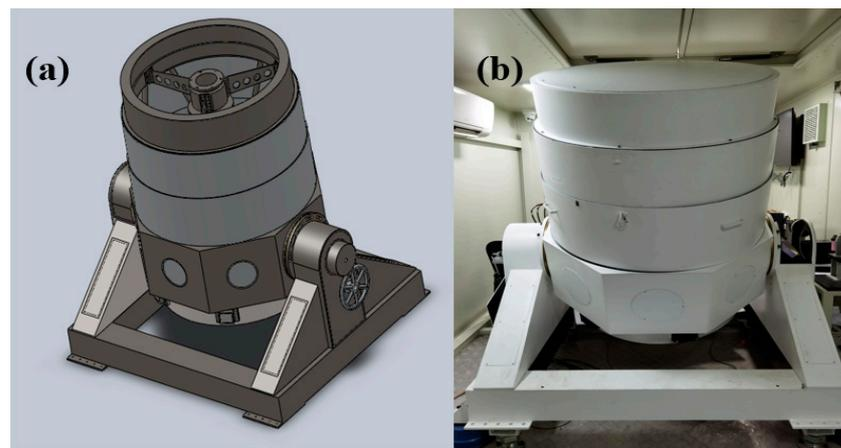
**Figure 13.** The structural of the upgraded 800 mm Cassegrain telescope. (a) Design diagram (b) Solid diagram.
