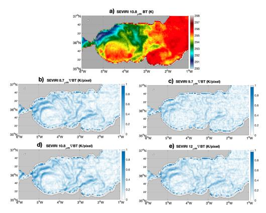
**Figure 6.** (a) TOA radiances for SEVIRI channel 9. (b–e) Sobel spatial gradients of the TOA radiances for channels 7 to 11. The fields refer to 5 August 2021 at 09:00 UTC.
