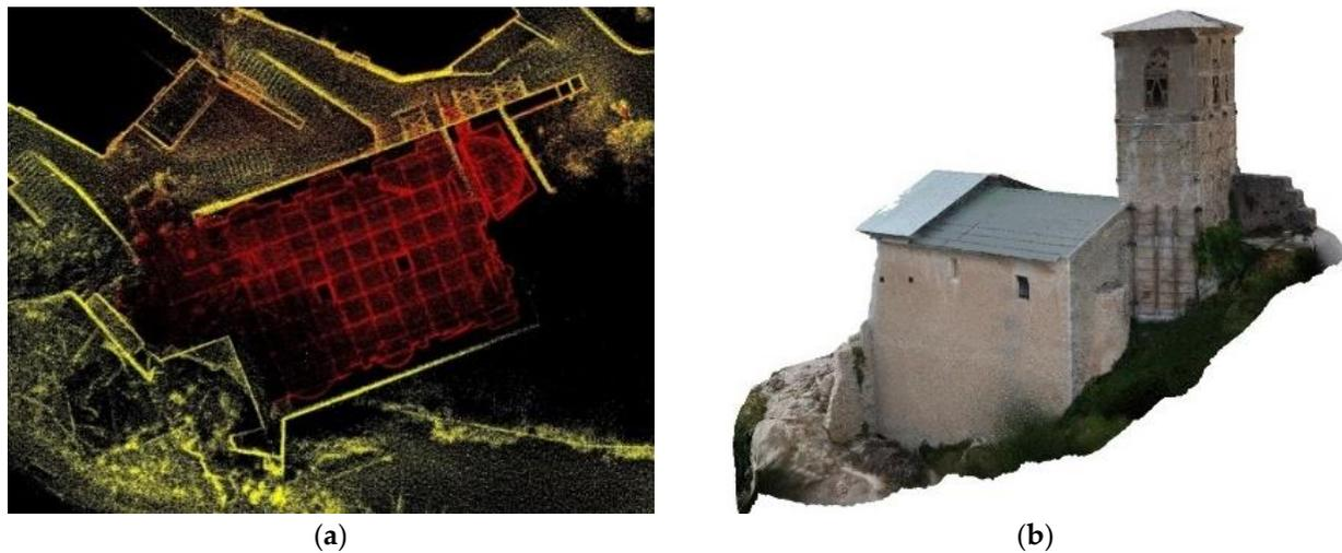
**Figure 4.** (a) Integration in planar view of indoor point cloud from mobile laser scanner (red) with outdoor point cloud from mobile scanner and UAV photogrammetry; and (b) textured 3D mesh model from UAV images data.
