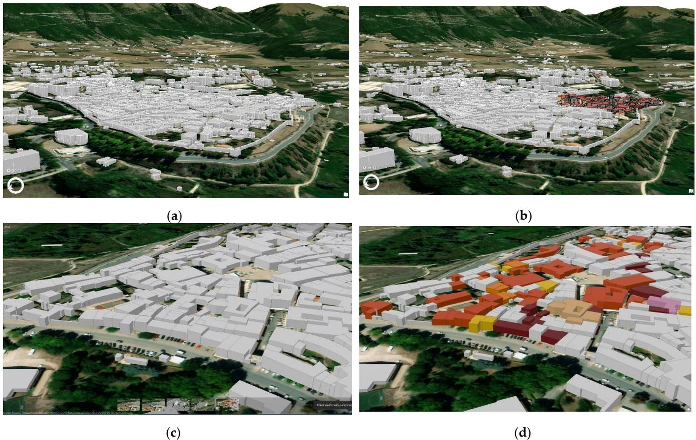
**Figure 7.** The LoD 1 3D model generated from urban cartography in GIS interface: (a) neutral representation; and (c) its zoom; (b) multi scale view with the LoD 3 modelled part on background; and (d) thematic mapping according to the attribute related to damages (AeDES reports).
