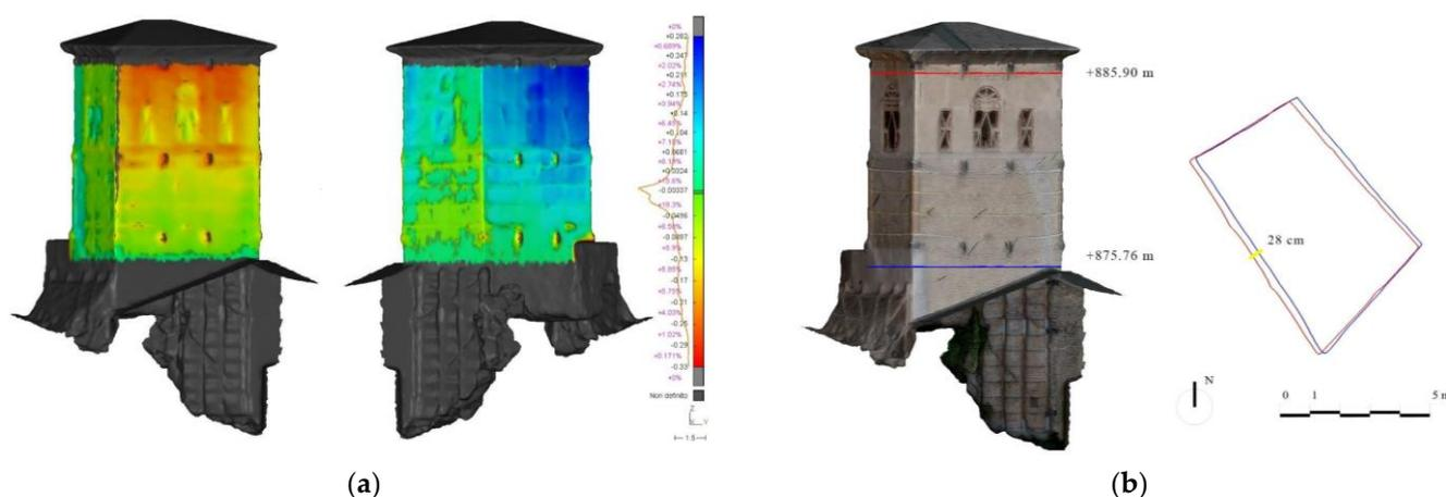
**Figure 15.** (a) Deformation evaluation based on the 3D mesh model with deviation analysis between the tower mesh and the profile at the base extruded along the vertical, underlining the off-lead of the bell tower; and (b) mesh profile at the base (blue) and mesh profile at the top of the tower (red).
