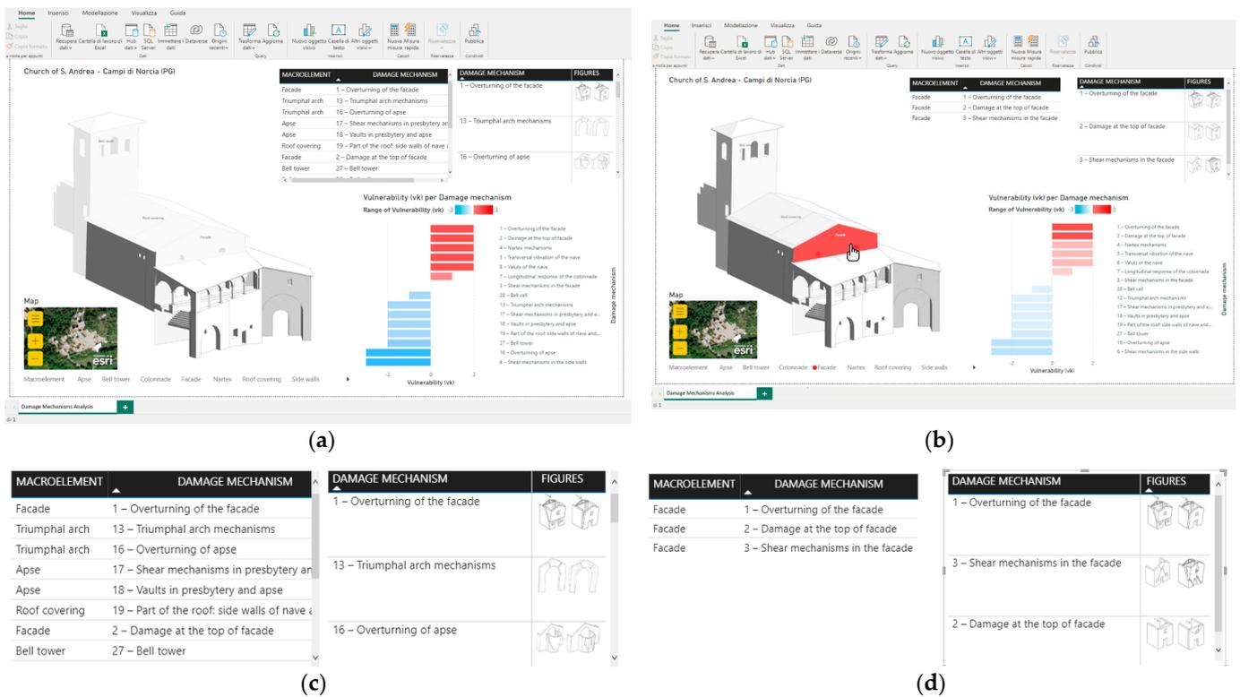
**Figure 19.** Thematic and interactive dashboard of S. Andrea’s Church damage mechanism: (a) general view with active tools, and (b) query of the façade element. In (c,d) respective zoomed view of the data reporting on the dashboard.
