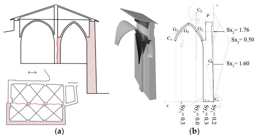
**Figure 16.** Representation of the wall mechanism: (a) 2D and 3D model extrapolated from the simplified volumetric; and (b) analysis of the south side wall, with graphical solution of the equilibrium conditions analysis for the calculation of the seismic coefficient.
