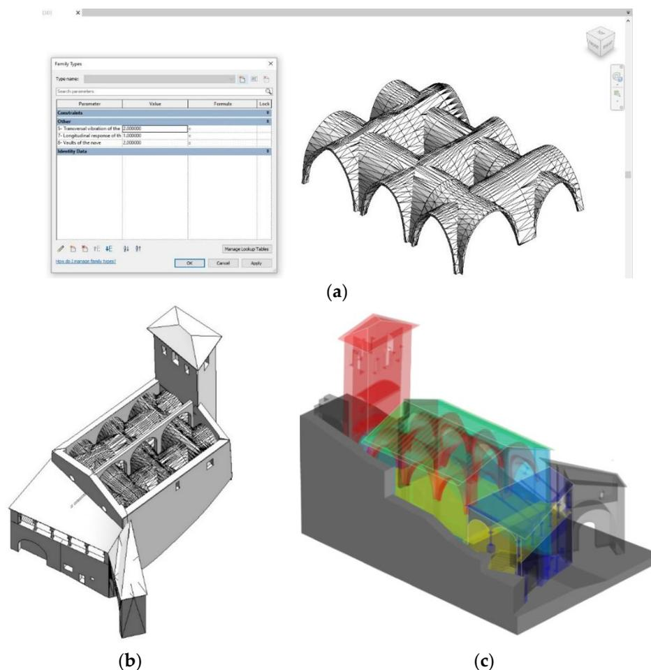
**Figure 13.** The as-built modeling steps for deriving accurate surfaces from point clouds. (a,b); and final microelement 3D volumetric model (c).
