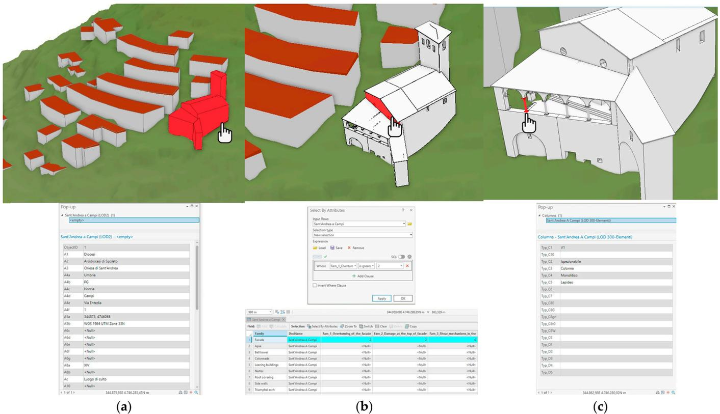
**Figure 18.** (a) Campi LoD 2 GIS model: the ground from DSM, LoD 2 buildings from matching point cloud and 2D shape file and georeferenced LOD 2 model of the church; (b) the LoD 3 church model where macro-elements were modelled from BIM, and damage mechanism information was associated; and (c) the LoD 4 church model where all elements were modelled, and information C and D were associated.
