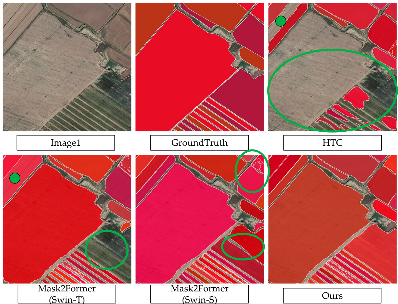
Figure 7. Visualization results of different models on fields with large-scale transformation. Green circles highlight areas of poor extraction.
