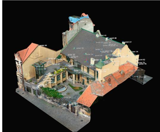
**Figure 5.** The use of control points in the Reality Capture program for the conformal alignment of photos in a single reference space.
