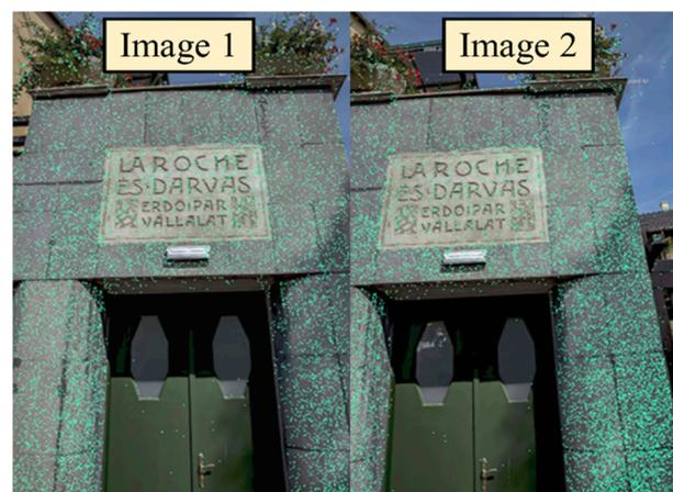
**Figure 6.** Identifying the points of connection in successive images following the processes of aligning the photos.
