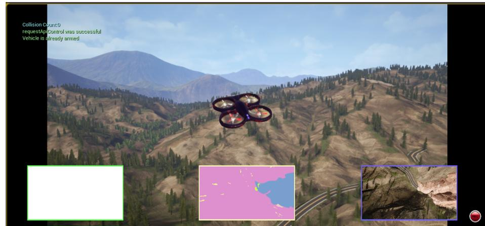
**Figure 3.** An example of virtual drone flight simulation within the proposed simulation framework (windows below, from left to right, show the depth map, semantic segmentation map, and photographic image).
