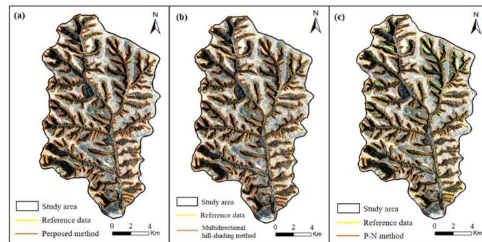
**Figure 16.** Extraction results of the shoulder line with the three methods: (a) proposed method; (b) multidirectional hill-shading method; (c) P-N method.
