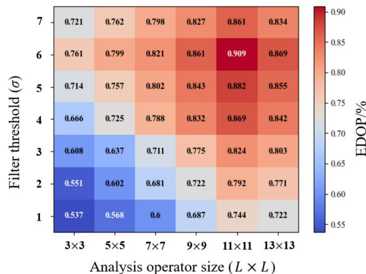
Figure 15. Two-factor heatmap of the effect of different values of  $L$  and  $\sigma$  on the extraction accuracy.
