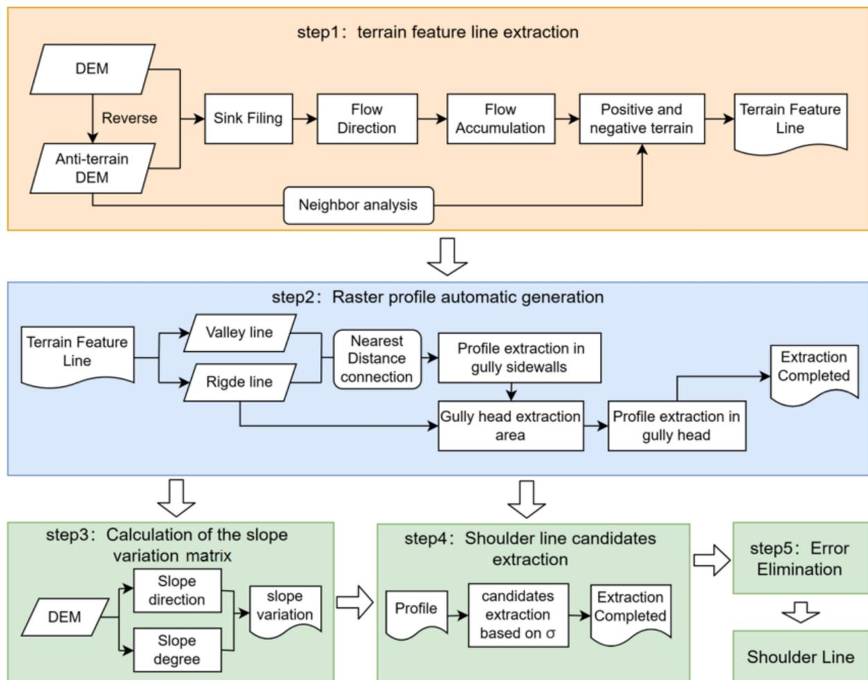
**Figure 5.** Automatic shoulder line extraction flow chart.
