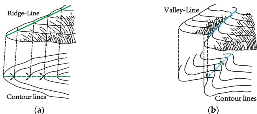
**Figure 6.** Schematic diagram of the terrain feature lines: (a) ridge line; (b) valley line.
