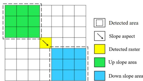
**Figure 9.** Analysis operator (size 7 \* 7 pixels).
