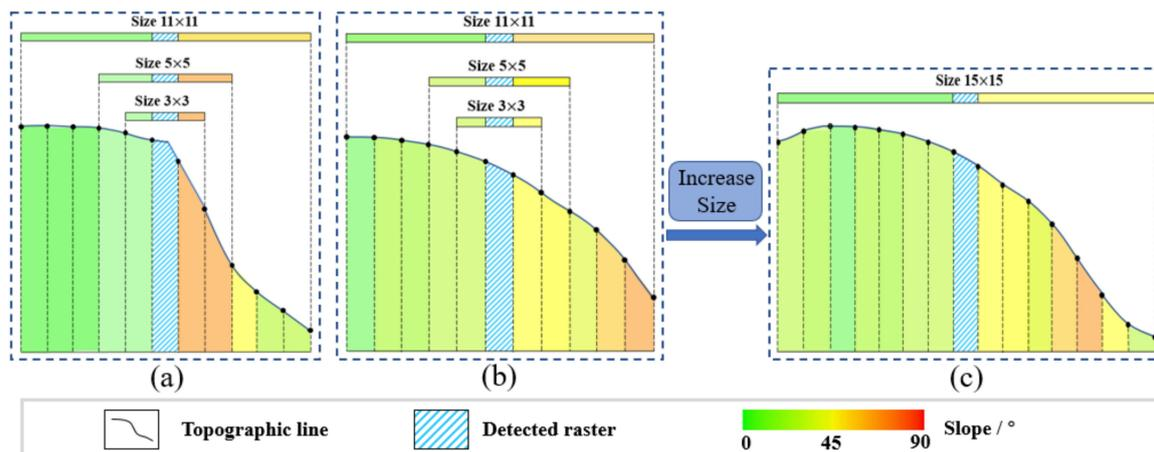
**Figure 14.** Influence of terrain factors on extraction: (a) areas with cliffs; (b) areas with gentle slopes; (c) areas with increasing size of the analysis operator.
