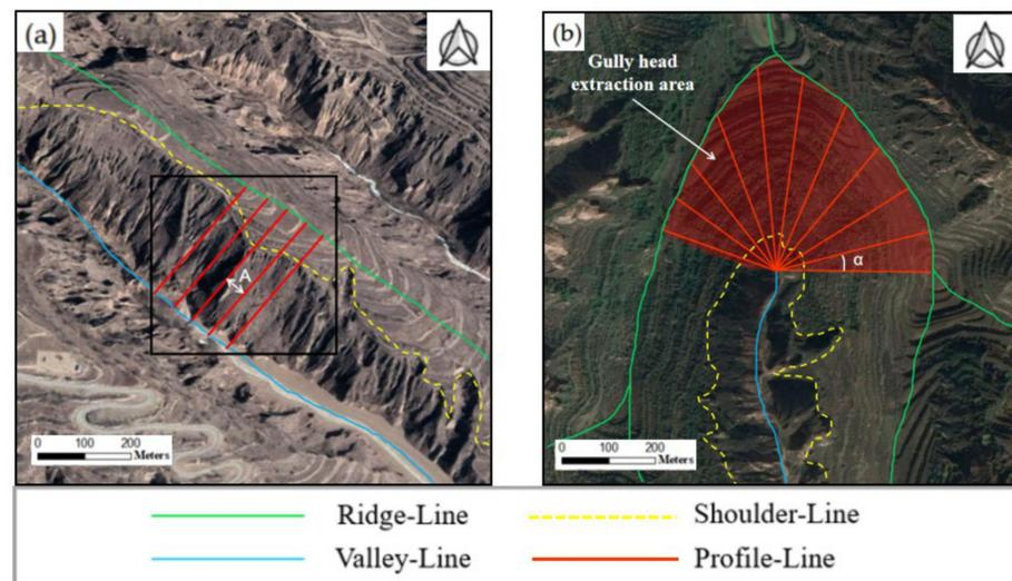
**Figure 7.** Schematic diagram of raster profile extraction: (a) at the gully sidewalls; (b) at the gully head.
