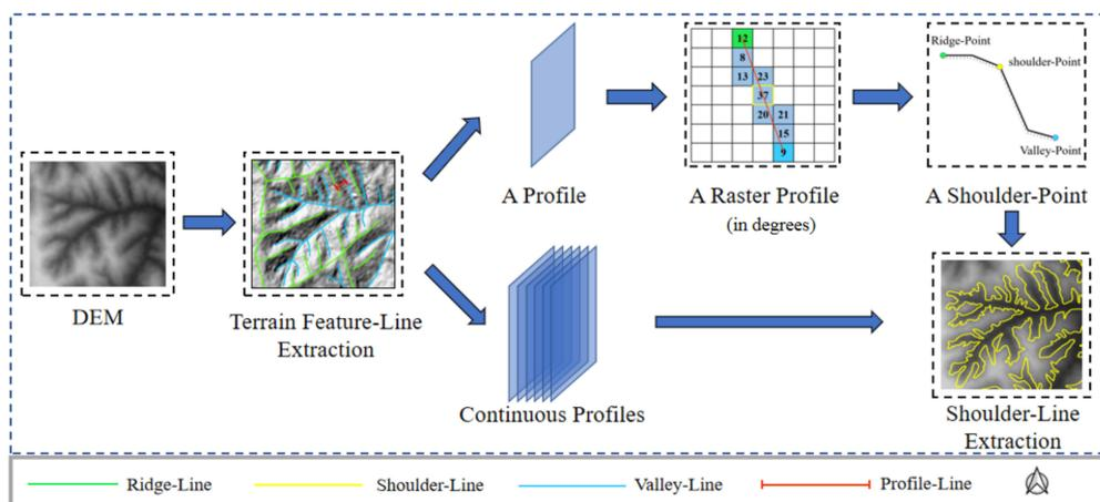
**Figure 4.** Flow chart of the principle of the automatic extraction of the shoulder line.
