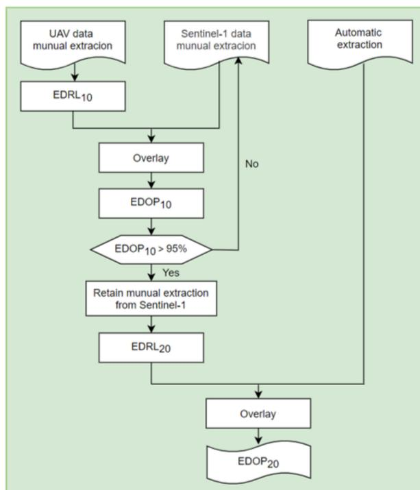
Figure 11. Proposed method of accuracy verification.
