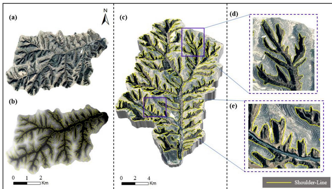
**Figure 12.** Result of automatic extraction: (a) remote sensing image map of the test area (acquired from Google Earth); (b) digital elevation model (DEM) of the test area; (c) 3D surface reconstruction of the test area; (d) jagged erosion; (e) palm-shaped erosion.
