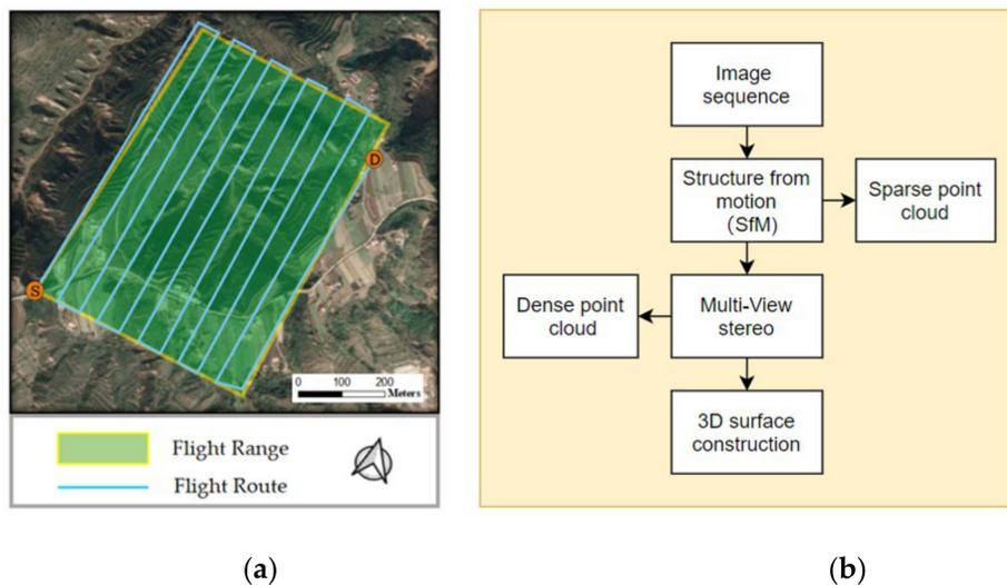
Figure 10. UAV data processing technology based on SfM-MVS: (a) route flight module; (b) SfM-MVS workflow.
