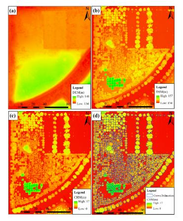
**Figure 5.** The DSM, DEM, CHM, and ITCD results: (**a**) DEM derived from UAV-RGB data; (**b**) DSM derived from UAV-RGB data; (**c**) CHM derived from UAV-RGB data; (**d**) ITCD results based on the watershed algorithm.
