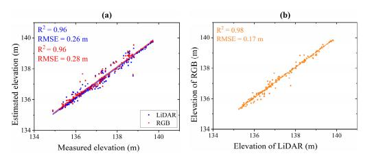
**Figure 4.** Correlation graph: (**a**) correlation between the field-measured elevation and the corresponding elevation values of  $DEM_R$  and  $DEM_L$ ; (**b**) correlation between the elevation values of  $DEM_R$  and  $DEM_L$ .
