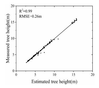
**Figure 9.** Correlation between the tree height after time difference correction and the tree height derived from UAV stereo images.
