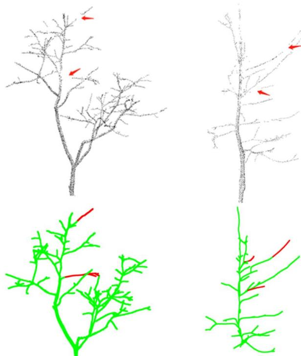
**Figure 17.** Skeleton completion effect. Red parts are the skeleton repair effect; green parts are the skeleton points.
